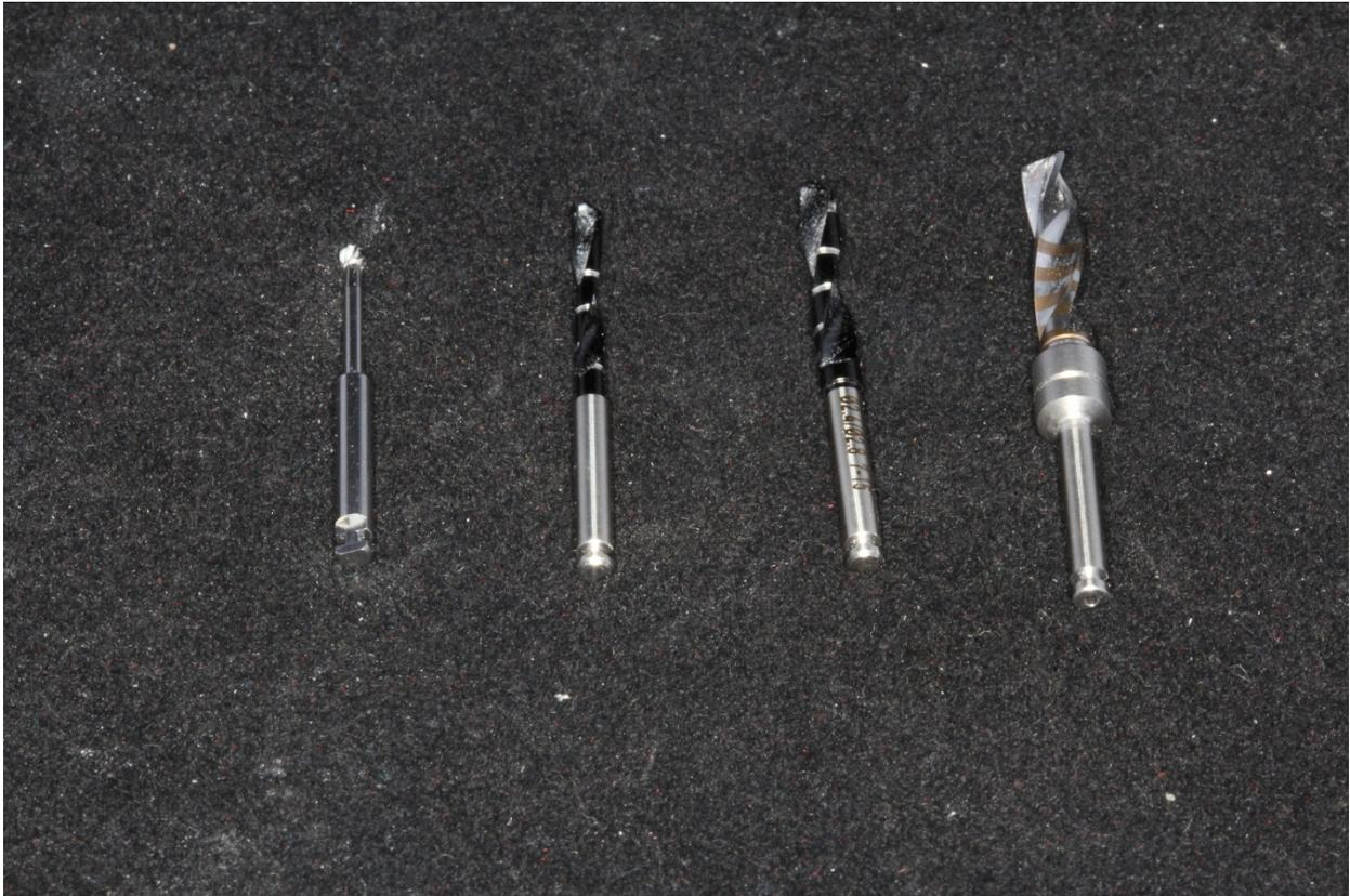
**Figure 9. Photo depicts drills used in this study. From left: 2 mm round drill, 2 mm twisted Drill, 2.4/2.8 x 7-15 mm twisted drill, 3.5 mm twisted drill.**
