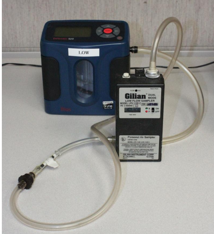
Figure 4: Calibration of a Gilian Pump Dual Mode Low Flow sampler Model LFS 113D using a Low Flow BIOS Defender Calibrator, Model 520-series
