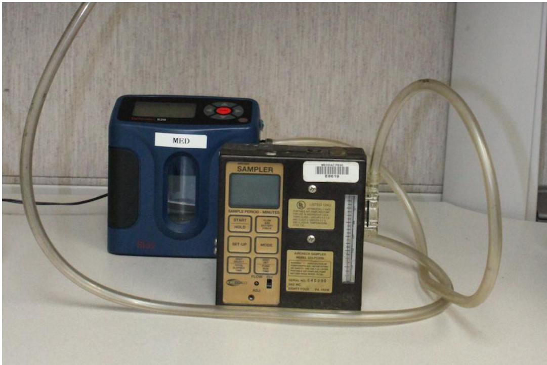
Figure 3: Calibration of SKC 224-PCXR4 using a Medium Flow BIOS Defender Calibrator, Model 520-series
