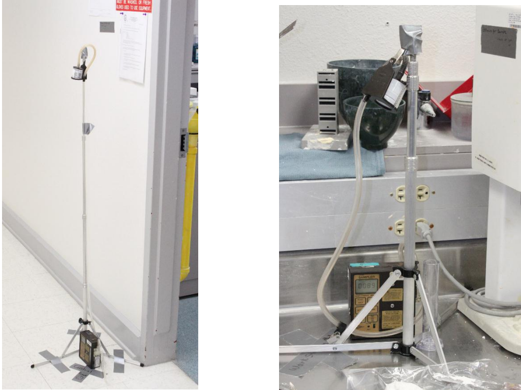
Figure 5: Real time particulate sampling in Hallway just outside of the lab and at workstation 1 near the stone distribution area
