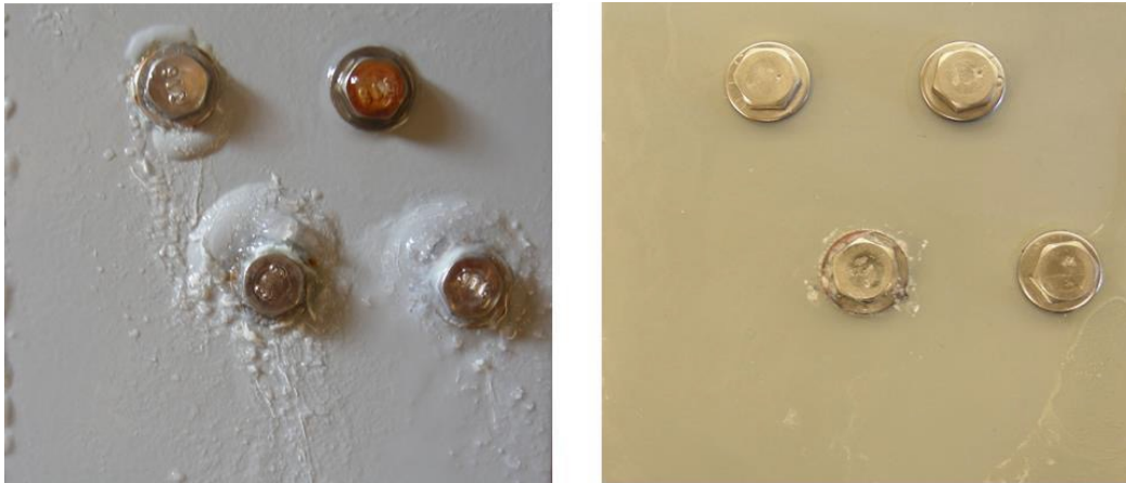
Figure 3: Photographs of non-chromated (left) and chromated (right) after 3 weeks exposure to salt spray fog.
