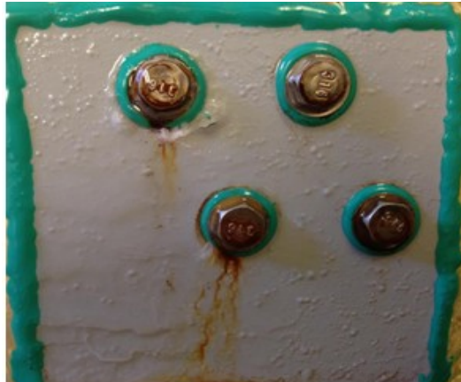
Figure 12: Image of galvanic panel with protected fastener holes after 180 days exposure to salt spray conditions.
