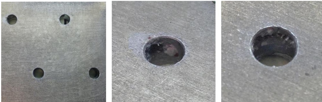
Figure 15: Images of sample with as-received hole condition after impressed current testing, showing damage induced to fastener hole wall during impressed current and no attack on top surface (left).
