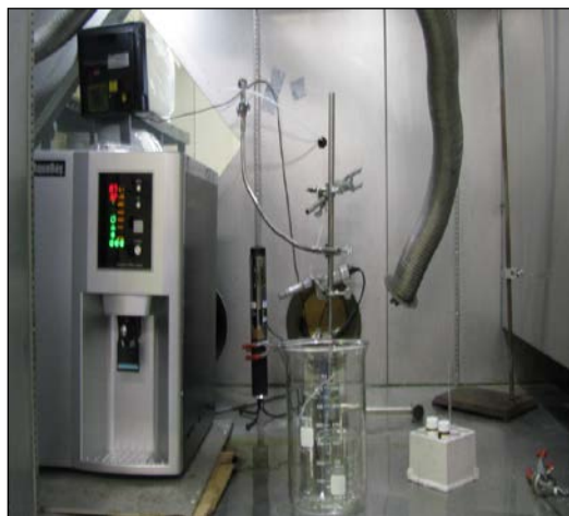
Figure 10. Environmental Chamber Set-up (2). Water from air system (left), control water (center) and benzene sampling vials (right)
