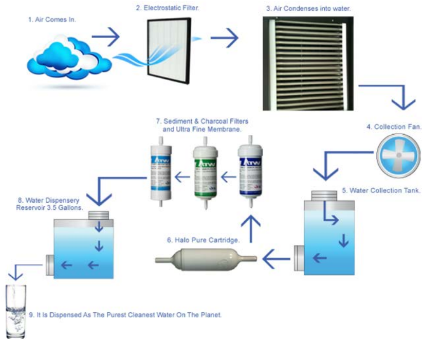
Figure 4. Manufacturer's Process Flow for the AquaBoy™ (4)
