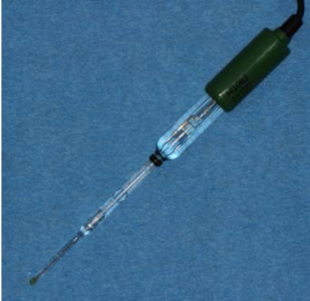
pH probe with micro bulb tip
