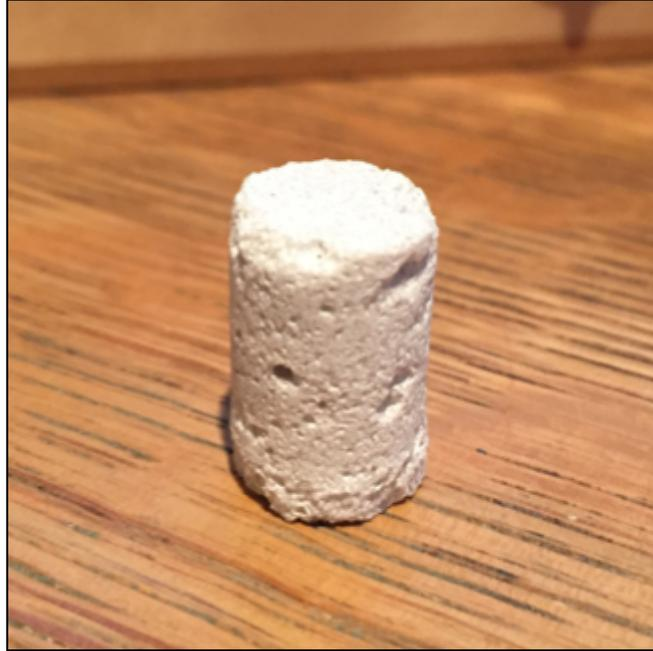
Figure 5: Image of titanium dioxide integrated concrete test puck (17.5 mm tall by 12.7 mm diameter) after testing
