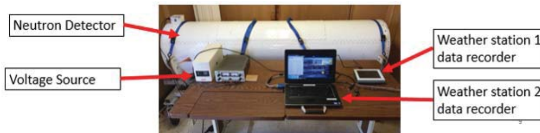
Figure 6.2: A look at the setup inside the satellite building. The LNS along the back wall, the computer connected to weather station 2, and the memory unit for weather station 1.
