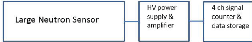
Figure 4.2: Block diagram of USNA detector
