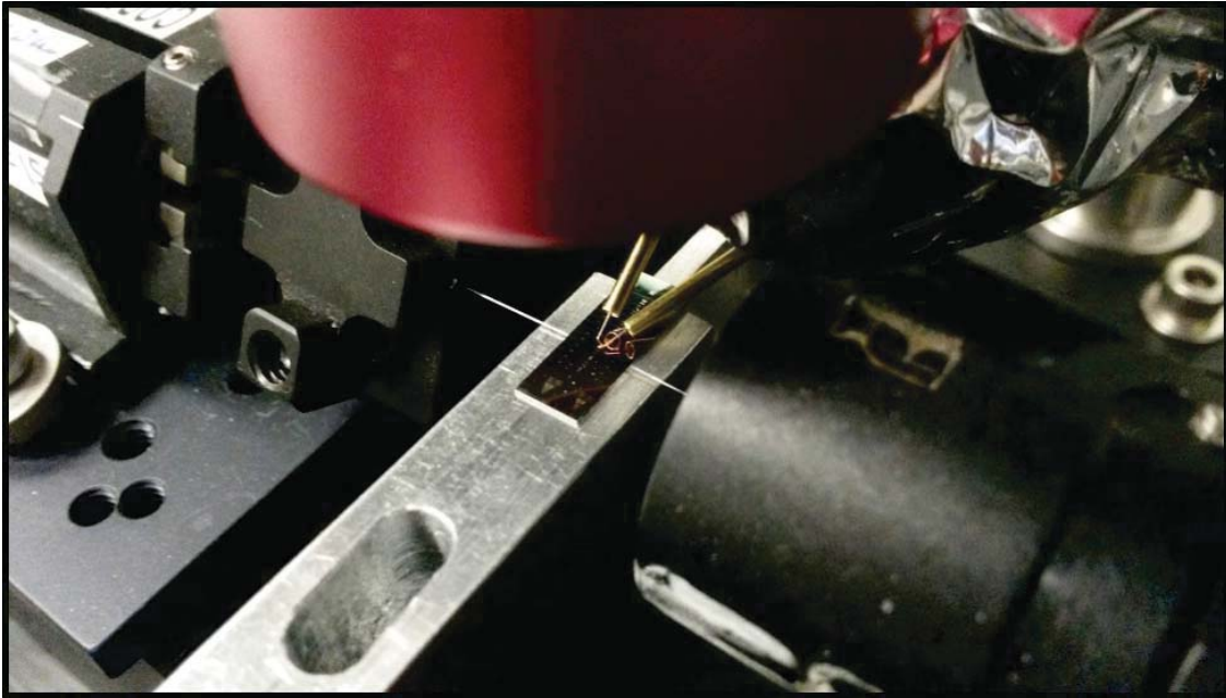
Figure 25: An image of the photonic integrated circuit with input and output lensed fibers coupled to the respective on-chip interferometer ports. Micrometered probes, monitored under a microscope (red objective) connected to a live video feed, are used to connect to the bridge electrodes in order to actuate the devices. The probes are encased in aluminum foil to avoid coupling unwanted ambient noise into the measurement.
