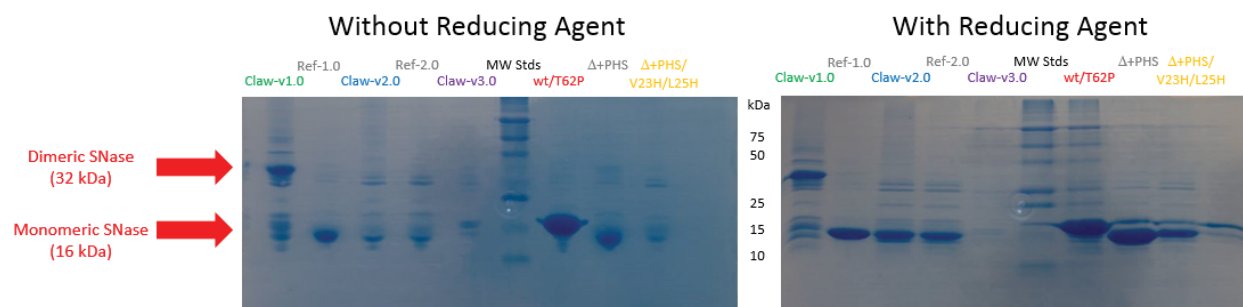
Figure 5: Denaturing electrophoretic gels of SNase variant proteins run in the absence (left) and presence (right) of the reducing agent, \beta -mercaptoethanol. Bands at 16 kDa indicated a monomeric protein. Bands at both 16 kDa and 32 kDa in the left panel suggested a disulfide-linked dimer formed between the single cysteine thiol from adjacent monomers in the Claw-v1.0 and Claw-v2.0 variants. Background proteins, \Delta +PHS, WT/T62P, Claw-v3.0 and V23H/L36H did not contain cysteine residues. Molecular weight standard masses are indicated.
