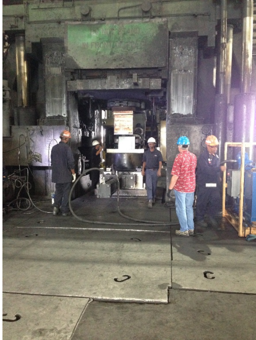
Fig. B-27 Insertion of the billet into the ECAE tool for the second pass. Note, the billet was turned on the round platform, shown in Fig. B-6, then picked up, and then lowered into the tool using the GLAMA manipulator.
