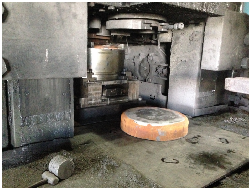
Fig. B-6 Front end of the ECAE tool already located in the press; the round platform was used to place and ease the rotation of the hot billet between successive passes, using the GLAMA
