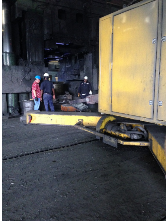
Fig. B-25 View of the GLAMA manipulator lifting up and holding a billet after the completion of the first pass
