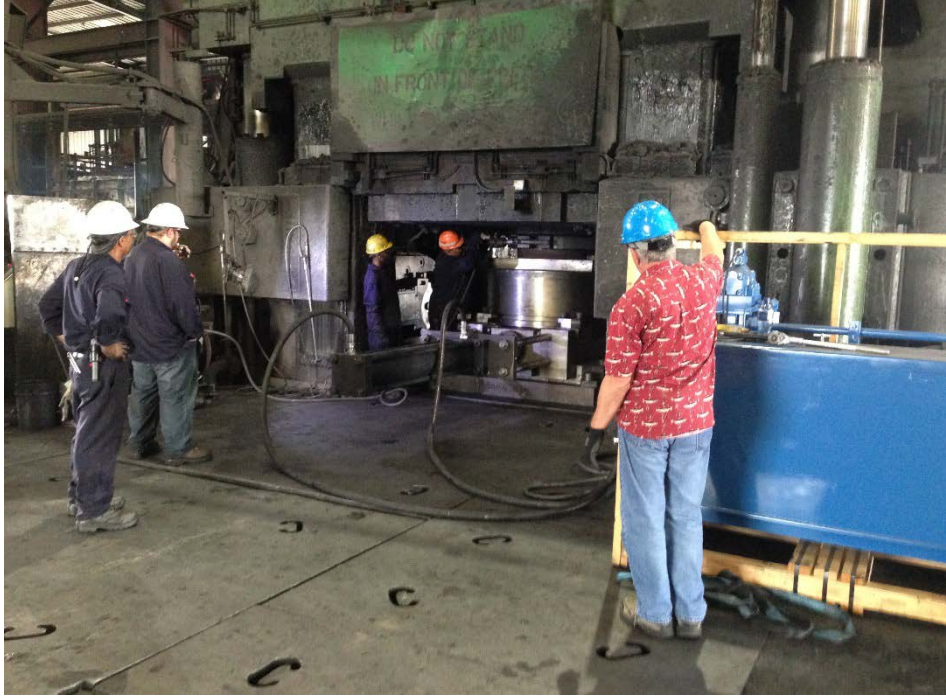
Fig. B-7 Punch fully inserted into the ECAE tool. Both of the hydraulic hoses, driving the backpressure system are already attached to the auxiliary power unit.
