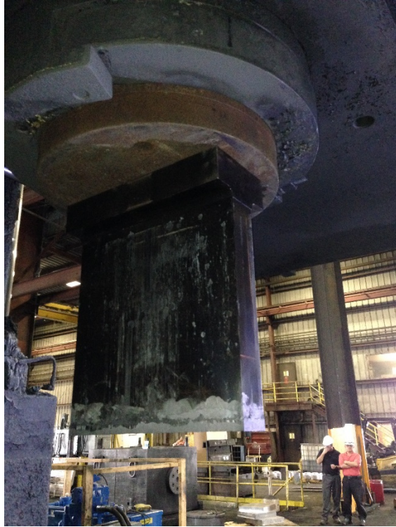
Fig. B-11 Close-up view of the punch. Note the anti-seize lubricating compound on its bottom
