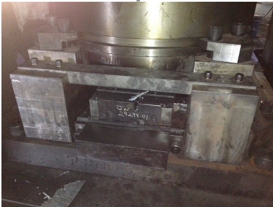
Fig. B-16 Close-up view of the front end of the tool with the bottom slider in the forward or ejection position
