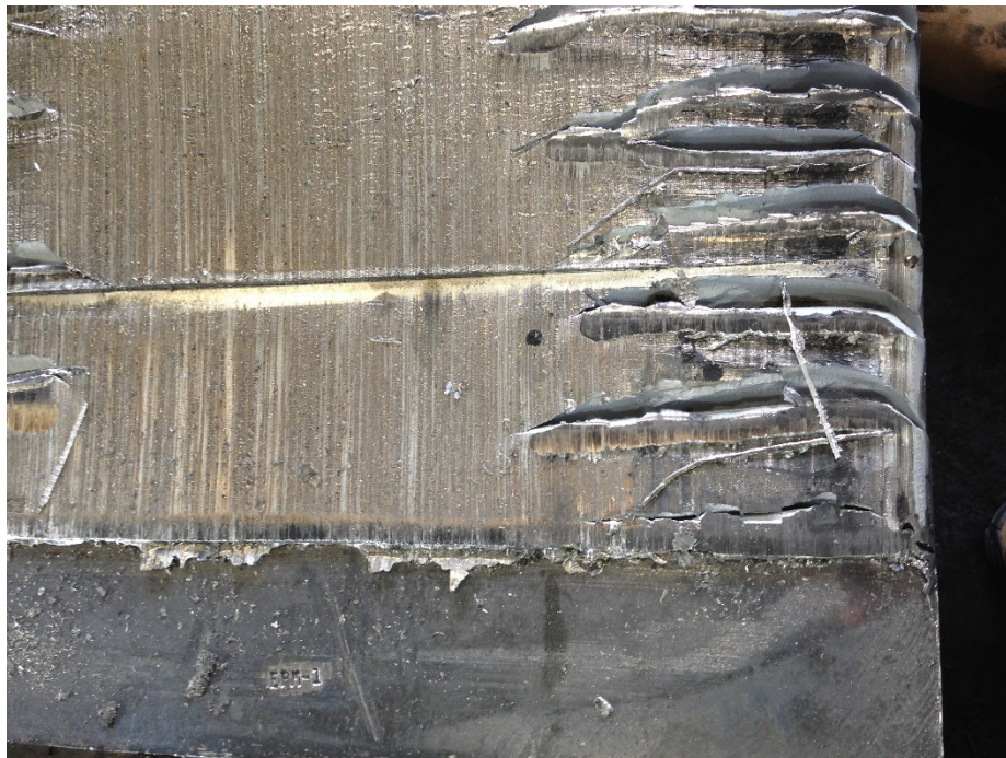
Fig. B-20 The 2-pass billet from Trial no. 1. Detail displaying the periodic lateral edge cracking in the billet; lower right-rear corner of the billet.
