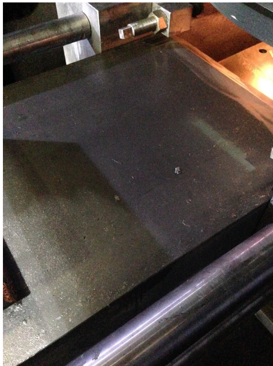
Fig. B-14 Close-up view of the bottom slider assembly. The bright orange light is caused by the ring heater inside the cavity.
