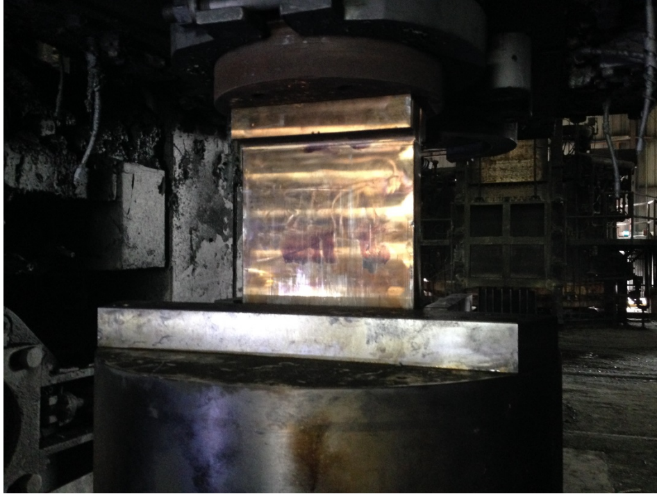
Fig. B-15 Close-up view of the punch partially inserted into the input channel
