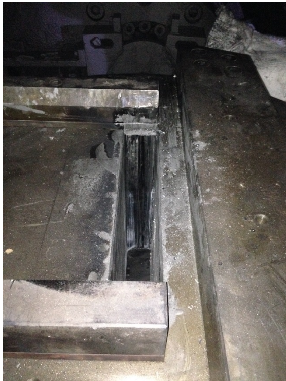
Fig. B-12 Close-up view of the top surface of the tool showing the rectangular input channel
