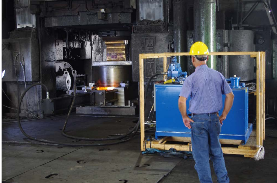
Fig. 6 Large-scale ECAE tooling die at the ETF 11,000-ton forging press with the auxiliary power unit on the right
