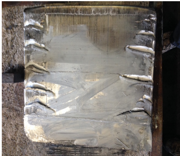
Fig. 8 Appearance of the ECAE processed billet after the second pass
