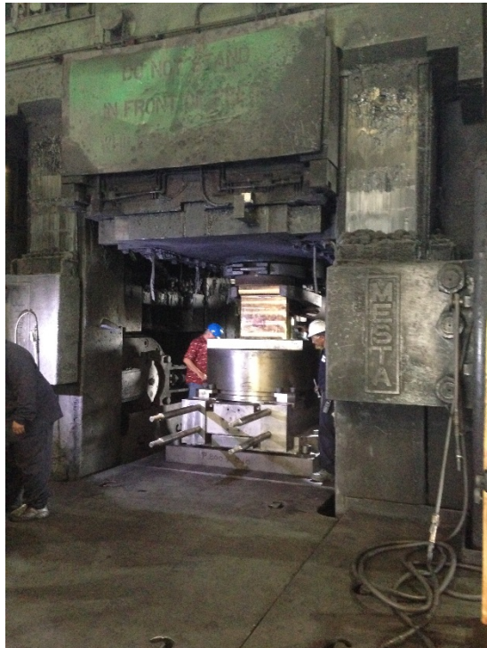
Fig. B-4 After loading, the ECAE tool had to be anchored to the floor of the forging press. During these adjustments, the punch is pulled out of the input channel.
