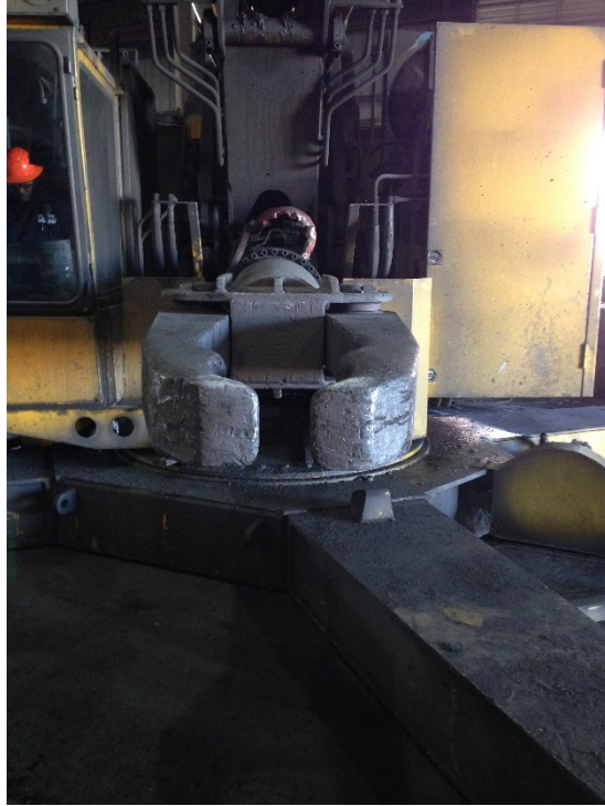
Fig. B-33 Close-up view of the manipulator mandible grip showing the potential difficulties in picking up and handling a rectangular billet with smooth surfaces
