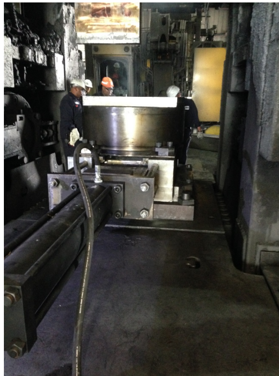
Fig. B-10 Close-up view of the hydraulic cylinder bolting arrangement attaching it to the base of the tool
