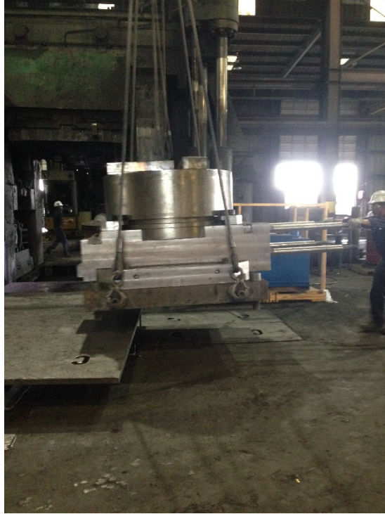
Fig. B-3 Side view of the ring and bottom assemblies of the ECAE tool being moved to the forging press by an overhead crane. The man on the right is included as a scale marker.
