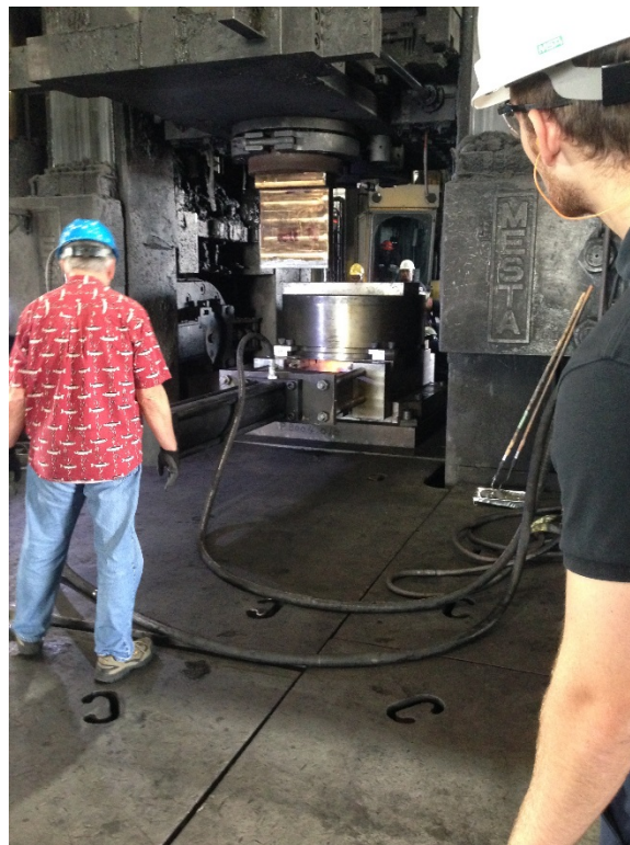
Fig. B-8 Punch has been retracted from the input channel of the tool and positioned to the side during additional preheating phase of the tool
