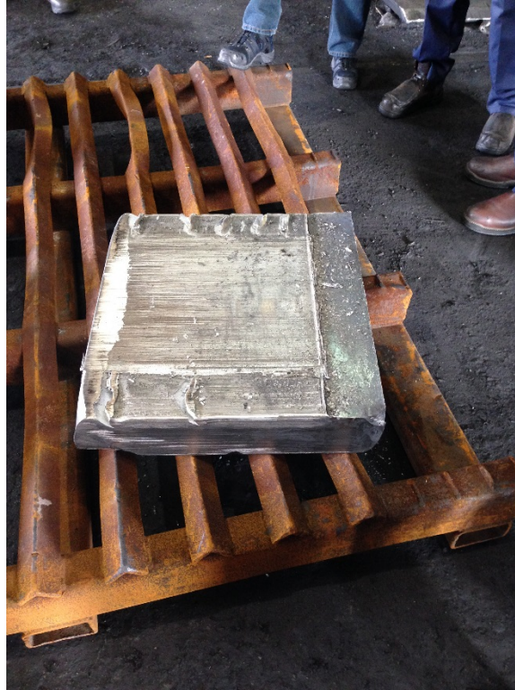
Fig. B-29 Side view of a 2-pass billet from Trial no. 2. Note the surface character of the cracks. Comparatively, these lateral cracks are fewer in number and not as deep into the billet as before.
