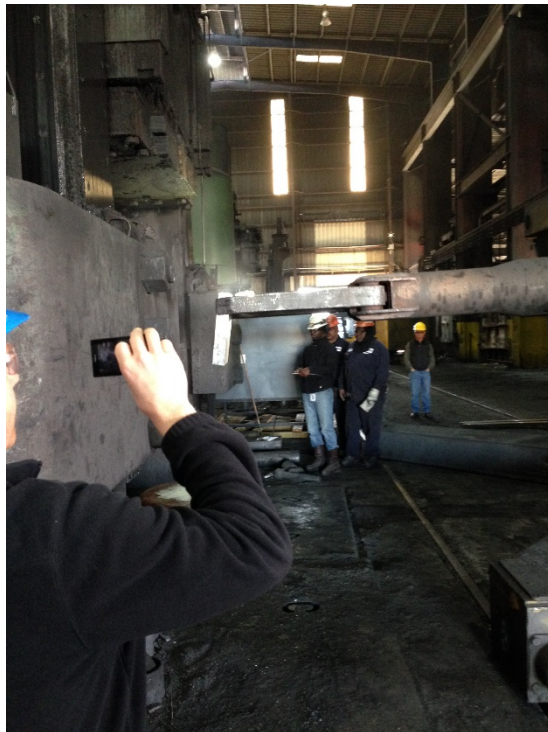
Fig. B-34 GLAMA manipulator grip mandible holding the hot billet in the vertical position and moving it over the ECAE tool for insertion
