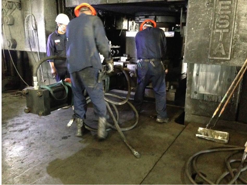
Fig. B-5 Attaching the hydraulic cylinder for the application of back-pressure and billet ejection control required some work
