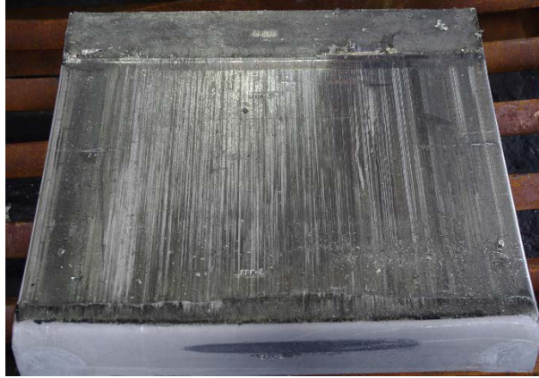
Fig. 7 Appearance of the ECAE processed billet after the first pass
