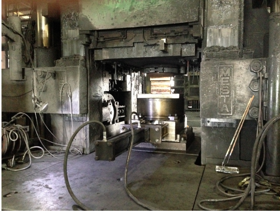
Fig. B-9 ECAE tool aligned and ready for operations
