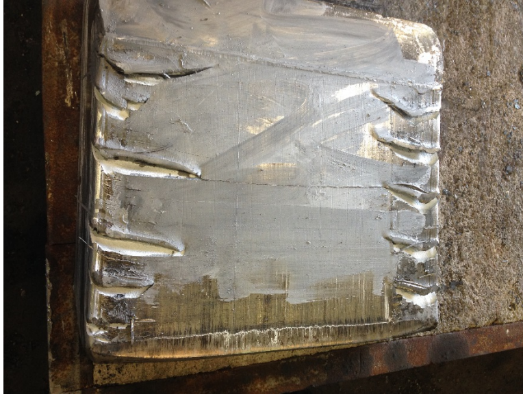
Fig. B 35 Side view of the second 2-pass billet from Trial no. 2. This billet exhibited considerably deeper and higher number of lateral cracks. The formation of the lateral crack was attributed to the reduced tool temperature.
