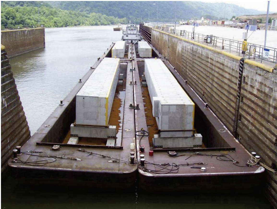
Figure 1.3. Marmet approach wall impact beam sections on barge for transport.
