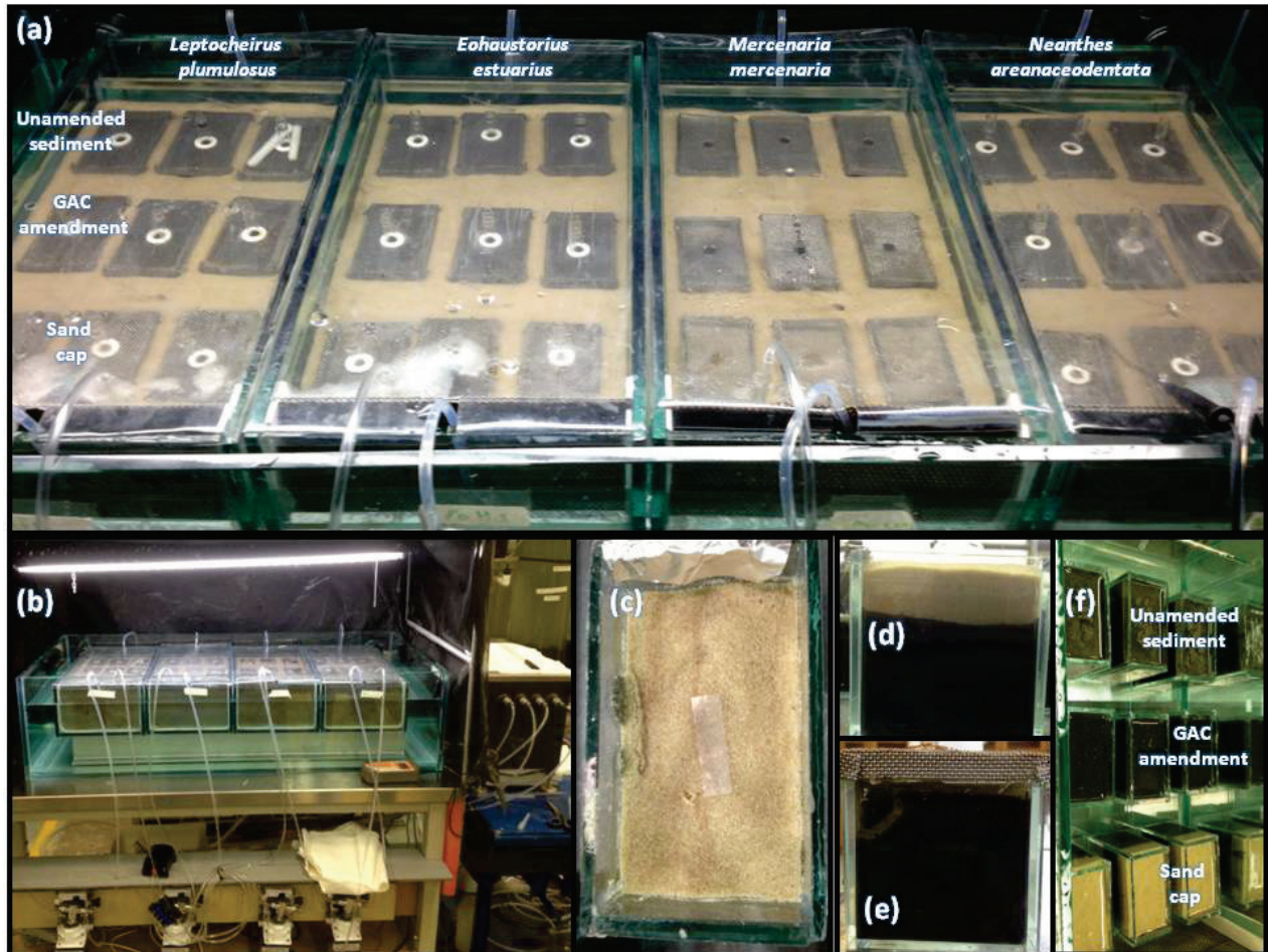
Figure 62. Photographs of the exposure system. Panel (a) illustrates the position of organisms and sediment amendments in the exposure system. Panel (b) shows the entire exposure system including pumps and reactors. Panel (c) shows the addition of a PED before the final 1 cm sand was added. Panel (d) shows a sand cap on top of the sediment. Panel (e) shows a Neanthes arenaceodentata burrow. Panel (f) shows the different sediment treatments prior to the addition of sand around the chambers.
