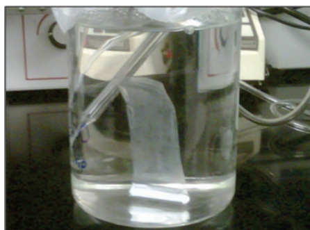
Figure 12. Experimental setup for SPMD-based passive dosing system.
