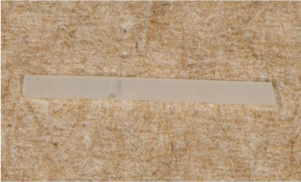
Figure 9. 1mm<sup>2</sup> Slab with defect from sectioning.
