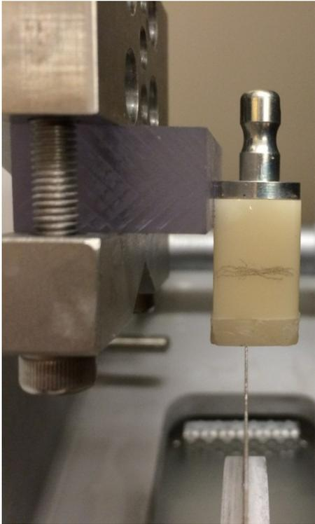
Figure 7. Block being sectioned with low-speed saw.
