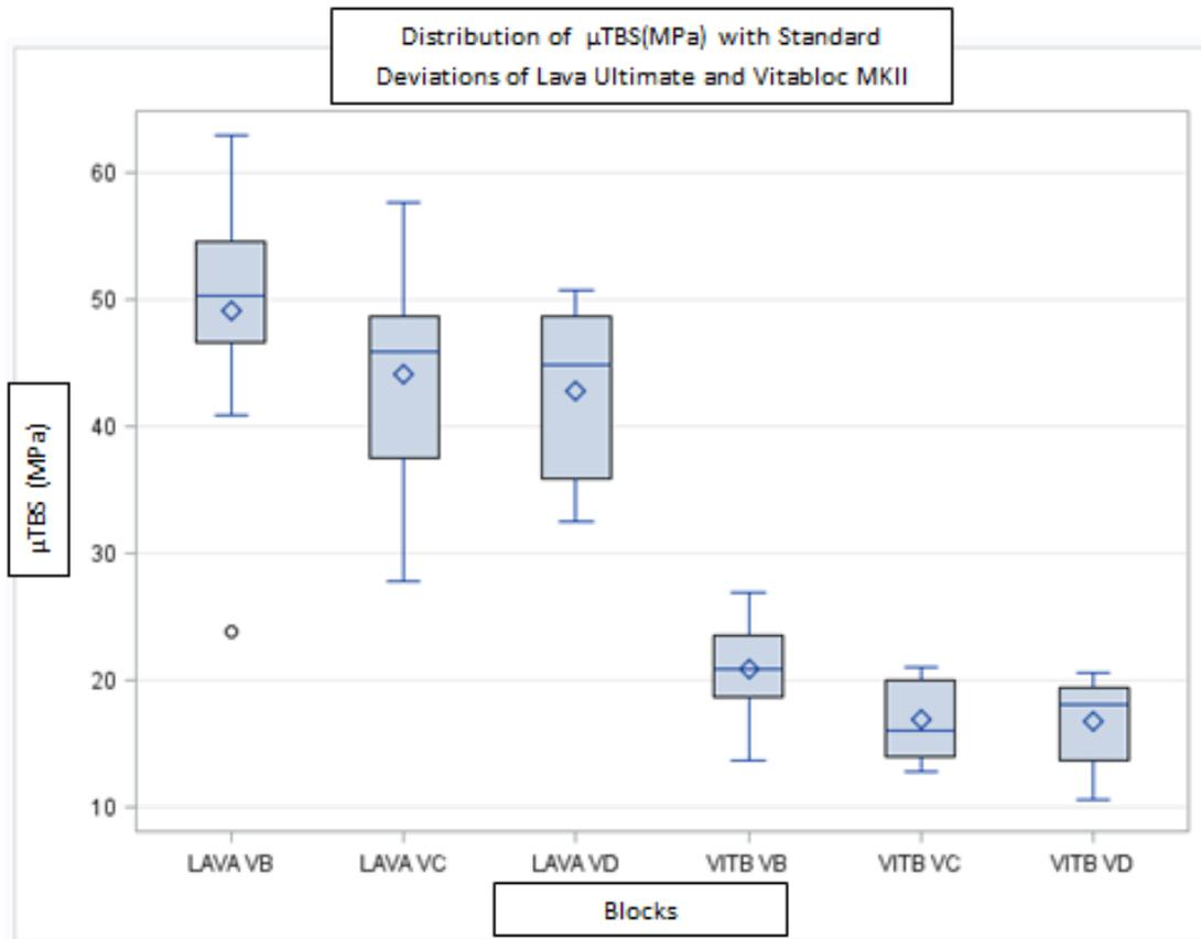
Graph 7. Distribution of mean  $\mu$ TBS within the blocks 'B-D'. The mean value of the blocks were not statistically different within the Vitabloc MKII or Lava Ultimate ( $P$  value  $> 0.05$ , Confidence  $>95\%$ ).
