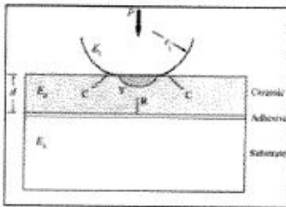
**Figure 1.** Schematic of brittle layer of thickness  $d$  and modulus  $E_c$  on a compliant substrate of modulus  $E_s$ , depicting sphere indenter of radius  $r_i$ . (Specimen radius  $r_s$  in general relation Eq. 1a is effectively infinite in the flat layer structure depicted here.) Damage modes: surface cone cracks (C); quasi-plastic yield zone (Y); inner-surface flexural radial cracks (R).
