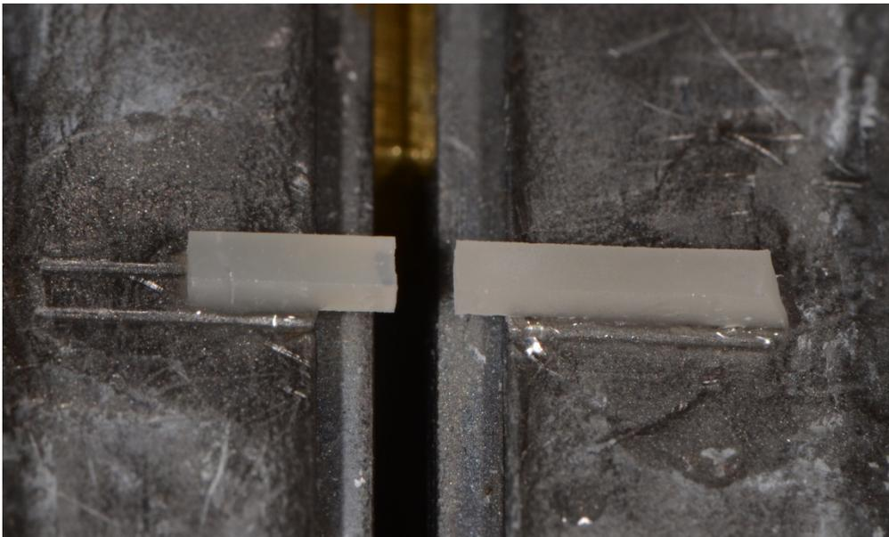
Figure 13. Lava Ultimate 1mm<sup>2</sup> slab demonstrating adhesive failure at the ceramic/cement interface.
