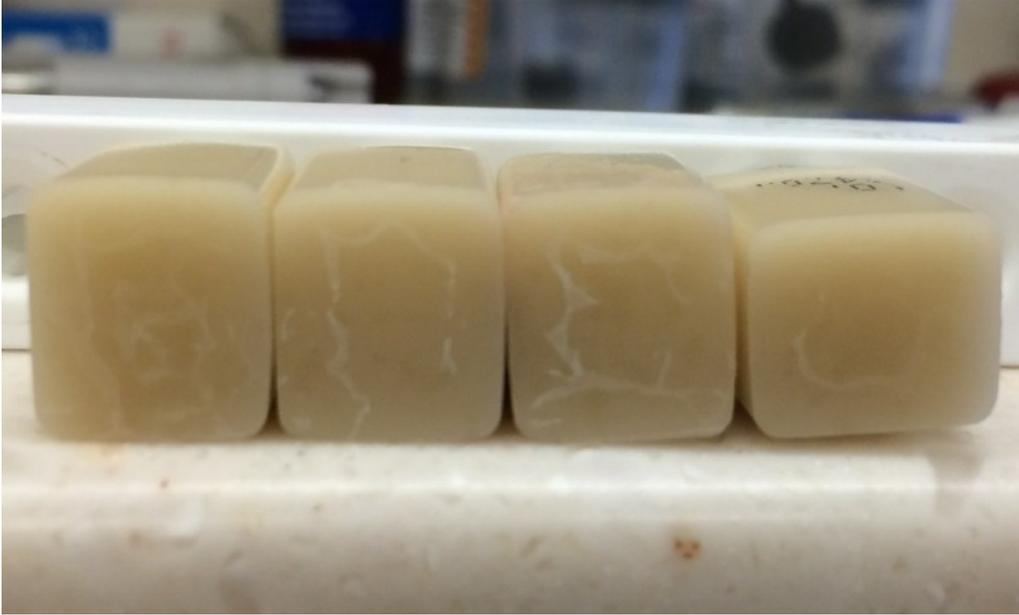
Figure 3. Vitabloc MKII blocks etched with hydrofluoric acid.
