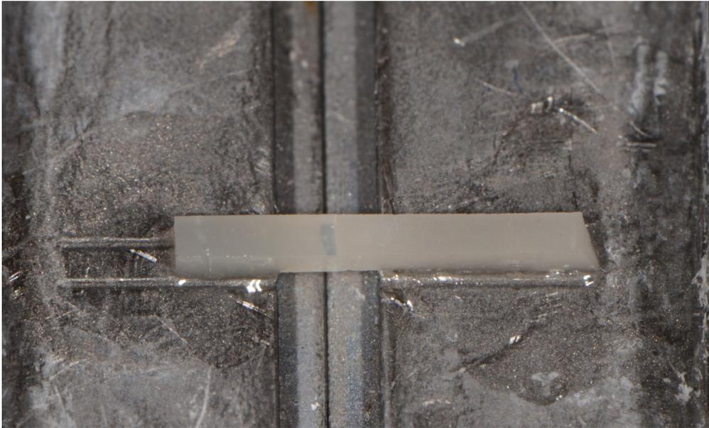
Figure 12. Lava Ultimate 1mm<sup>2</sup> slab with Z100 composite on left, cement layer in the middle, and Lava Ultimate on right.
