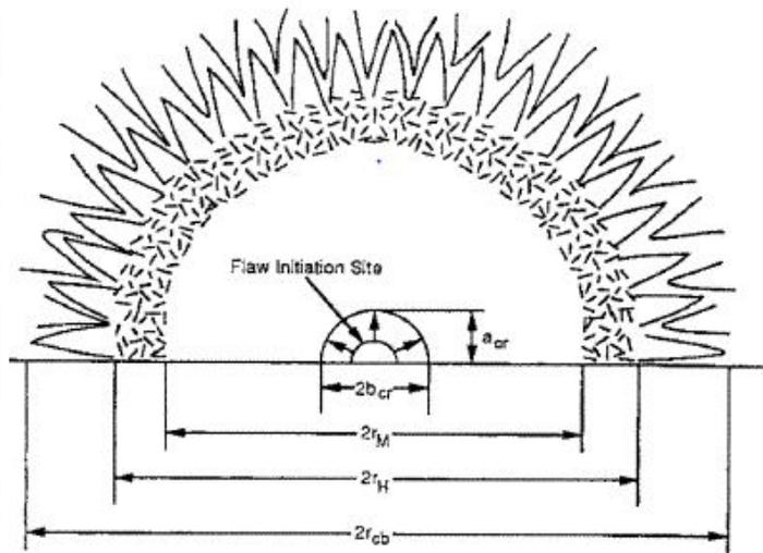
**Figure 1.** Schematic illustration of the fracture surface of a brittle material. Inner semi-ellipse represents the initial flaw, and outer semi-ellipse represents the critical flaw size. The subscripts M, H, and cb represent mist, hackle, and crack branching, respectively.
