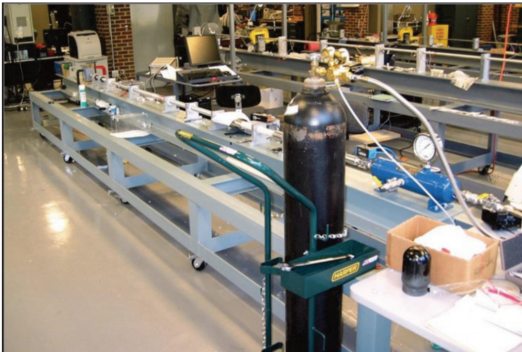
Figure 4-13. Compression SHPB setup at MSU CAVS.
