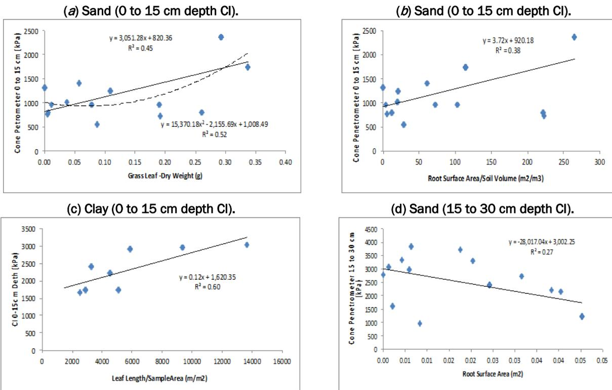
Figure 19. Godwin drop cone penetrometer measurements (Shoop et al. 2013).
