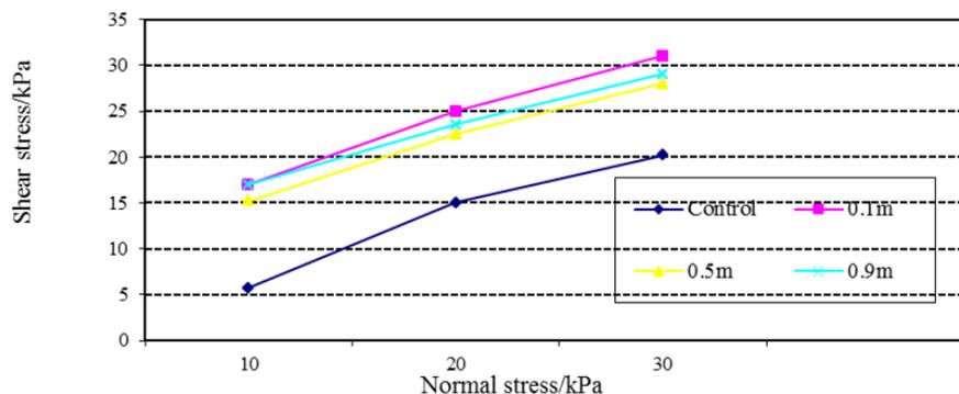
Figure 8. Values of cohesion ( $c'$ ) for vetiver-grass-reinforced soils at various depths. (Reprinted by permission from Ali and Osman 2008, Fig. 5.)
