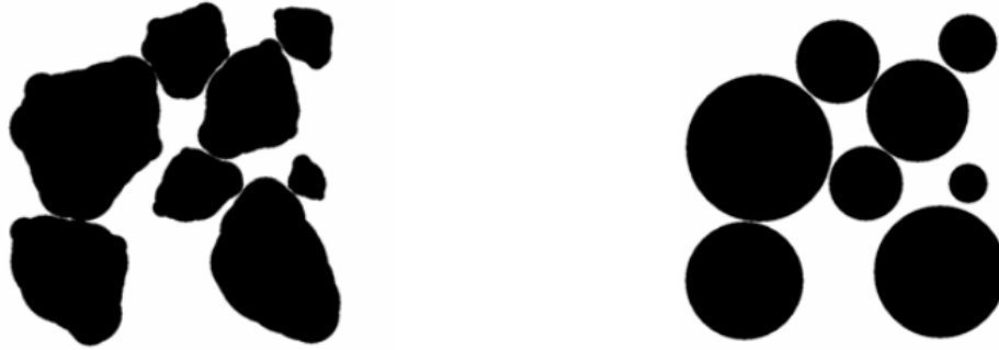
Figure A.36 Schematic of random assembly of eight angular particles (left) and transformed equivalent DSEs (right)
