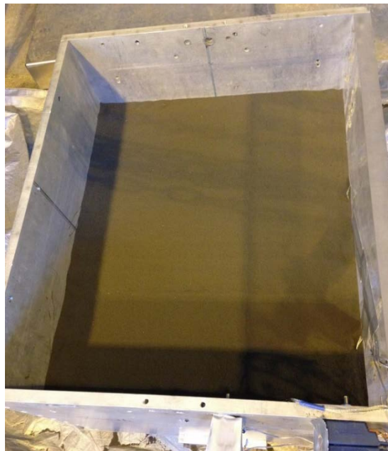
Figure 4.6 Surface of the granular profile after pluviation
