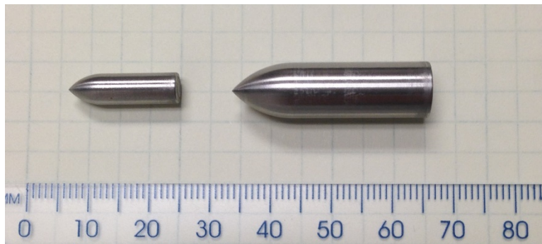
Figure 2.4 Photos of the projectiles used in centrifuge tests
