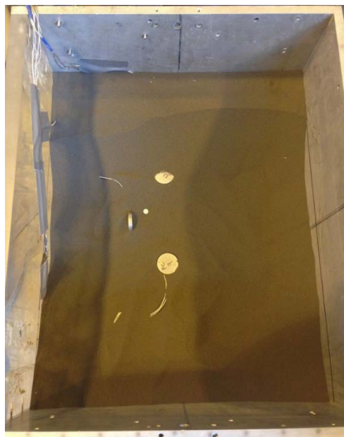
Figure 4.22 Relative position of the penetrated projectile with respect to the pressure cells (shown after test 3b)
