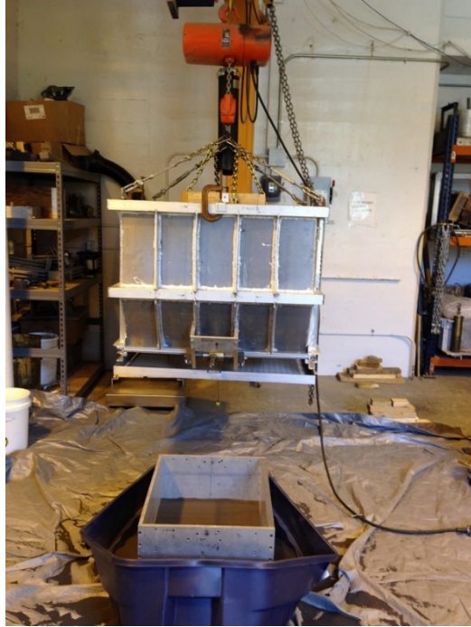
Figure 4.5 Pluviating proppant inside the rigid centrifuge container
