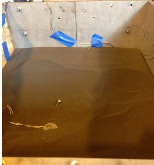
Figure 4.21 Profile after excavation at the end of test 3a
