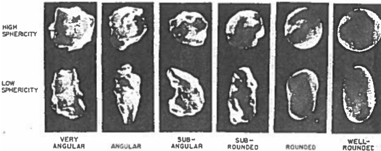
Figure A.24 Example of particle shape characterization (from Powers 1953): a) Roundness grades; b) Roundness scale
