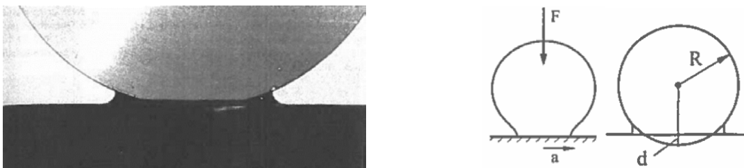
Figure A.10 Formation of a characteristic “neck” during adhesive contact (Popov 2010)
