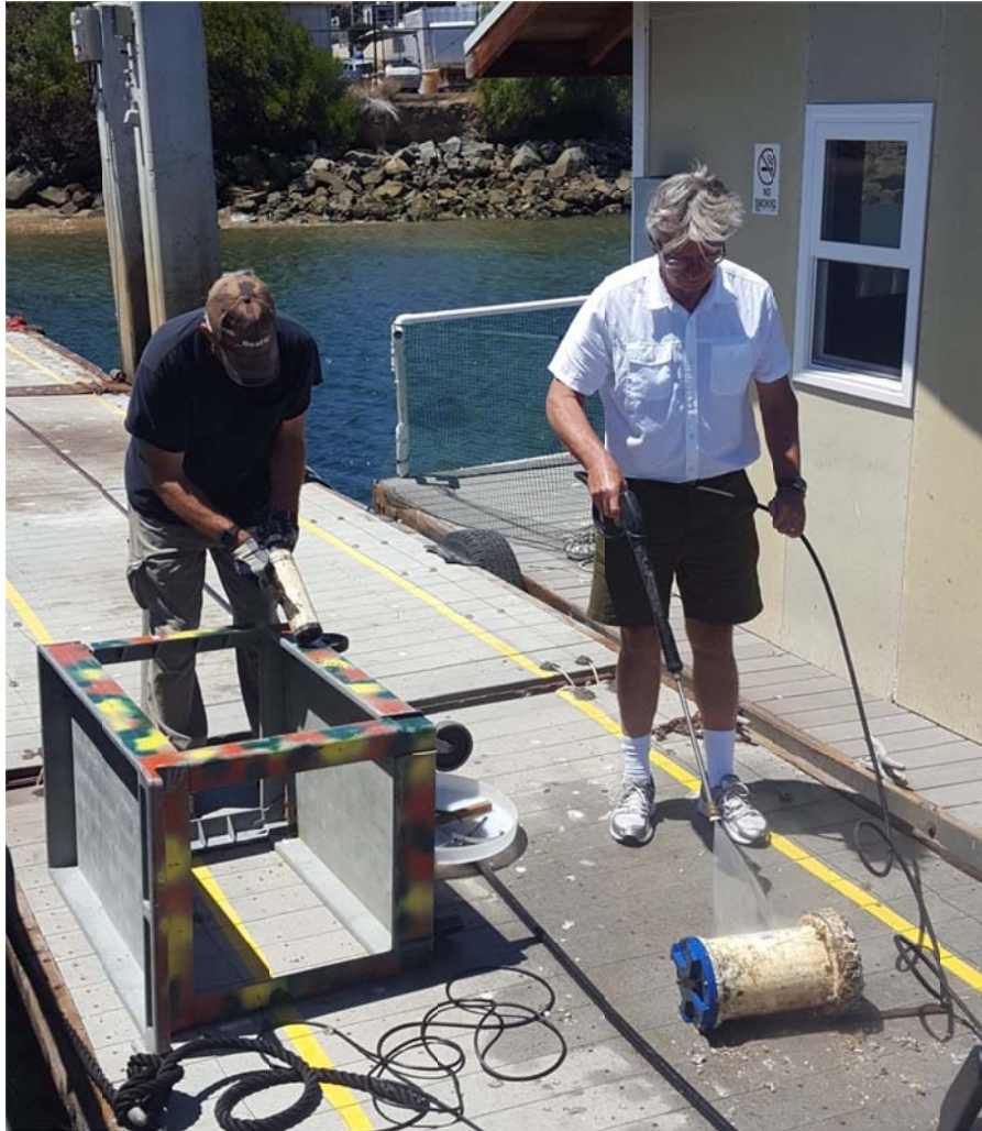
Figure 15. Removing biofouling from the ADCP and OBS instruments at the end of the RARA deployment on August 15, 2016.
