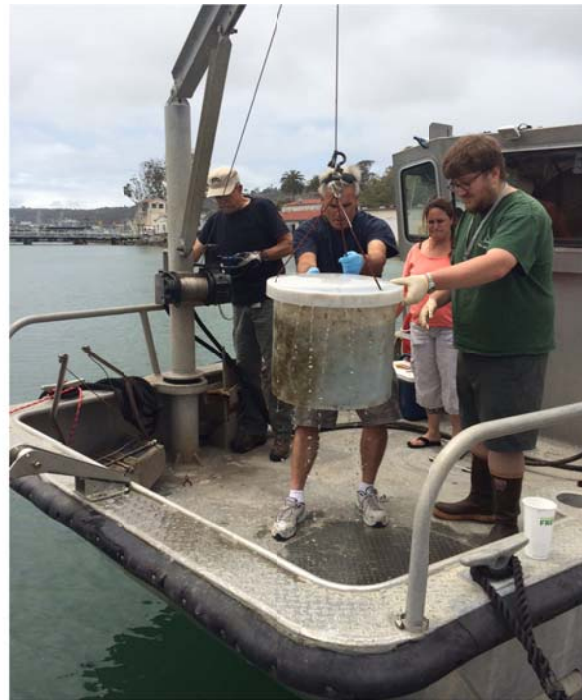
Figure 14. Retrieval of individual sediment cells during the May 24, 2016 (T-Mid) event.
