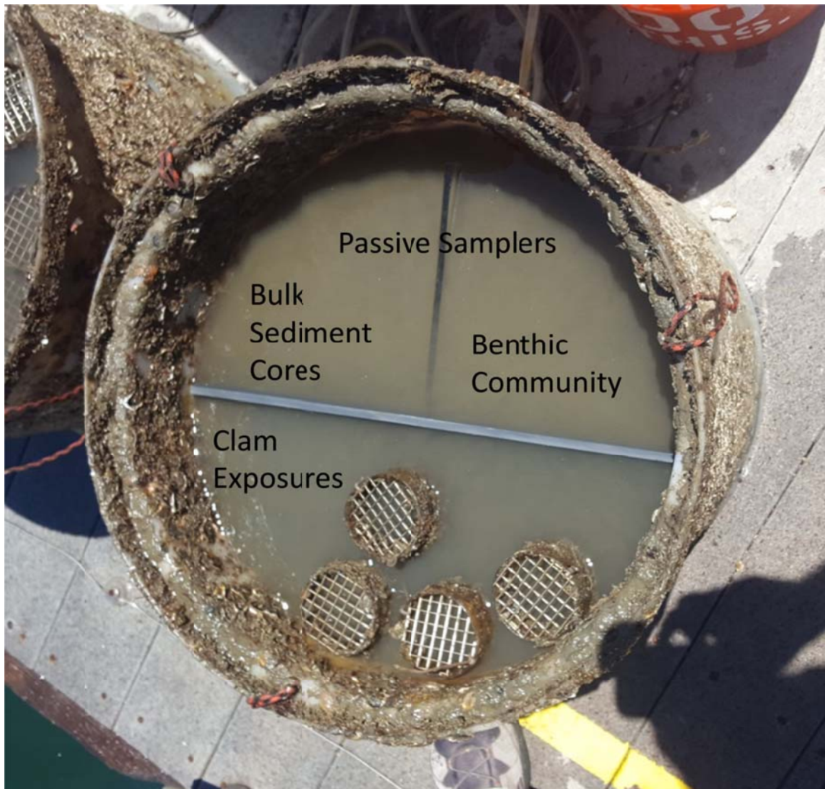
Figure 19. Photo from the August 15, 2016 event at the end of T-Final showing the segmentation of the RARA sediment cell into sampling zones for benthic community analysis, bulk sediment cores, and clam and passive sampler exposures
