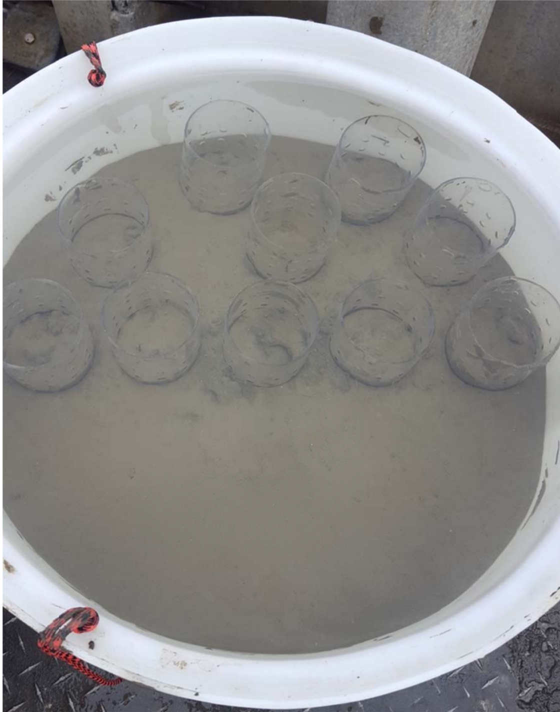
Figure 10. Final result for thin clean sediment layer treatment after final installation of treatment and overlying water.
