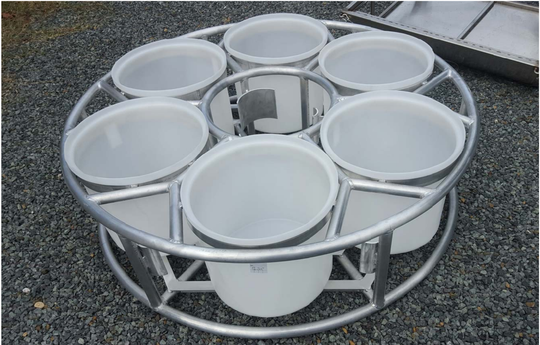
Figure 7. Photograph of the completed RARA frame during test fit of the sediment cells.
