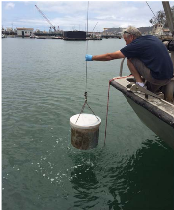
Figure 14. Retrieval of individual sediment cells during the May 24, 2016 (T-Mid) event.
