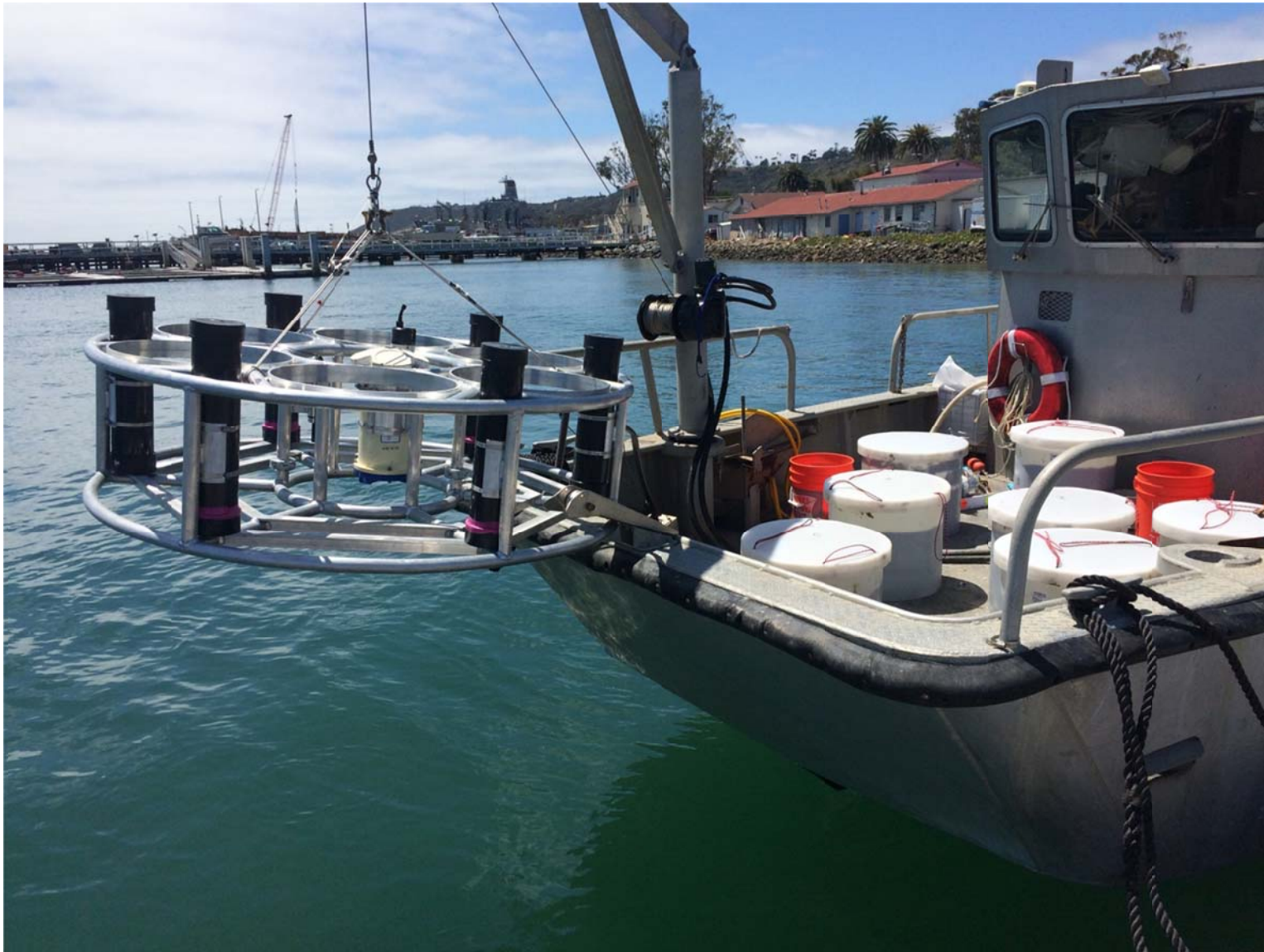
Figure 11. The RARA frame being deployed with sediment traps and instruments pre-installed from the R/V Ecos during the April 22, 2016 event.
