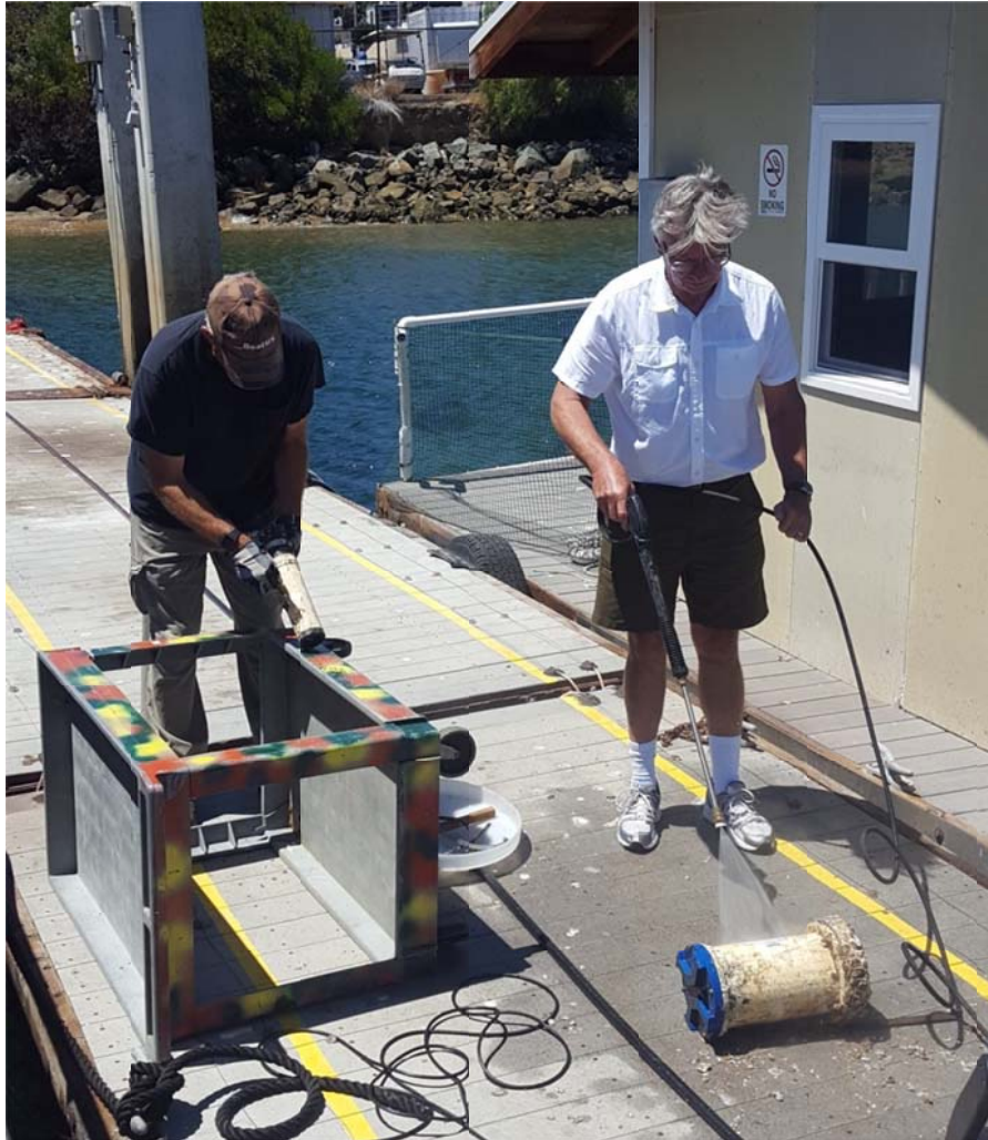
Figure 22. Removing biofouling from the ADCP and OBS instruments at the end of the RARA deployment on August 15, 2016.
