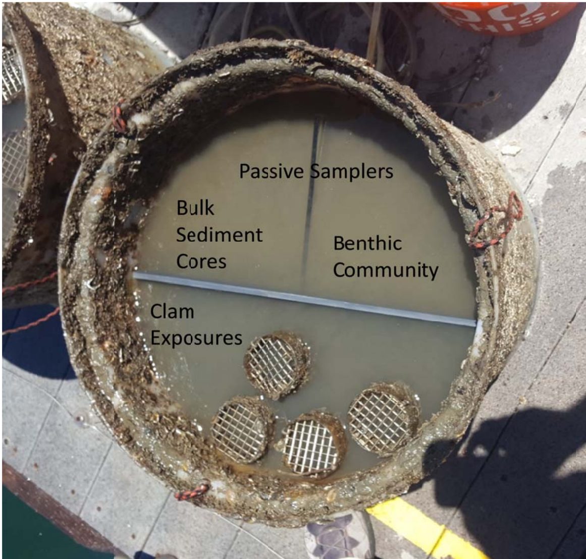
Figure 12. Photo at the end of a T-Final showing the segmentation of the RARA sediment cell into sampling zones for benthic community analysis, bulk sediment cores, and clam and passive sampler exposures.
