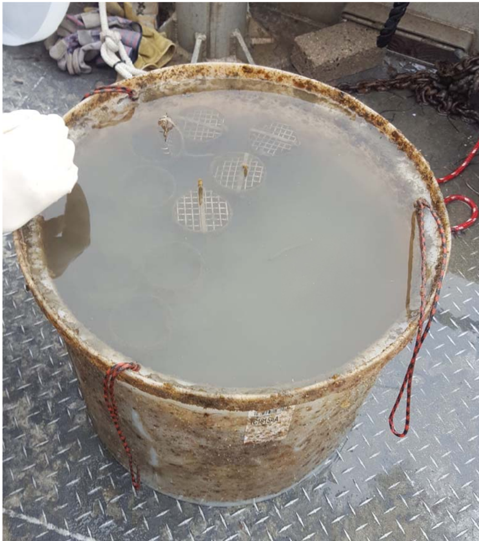
Figure 18. Preparing to remove clams and polyethylene passive samplers from a RARA sediment cell during the June 21, 2016 event at the end of the T-Mid exposure period.
