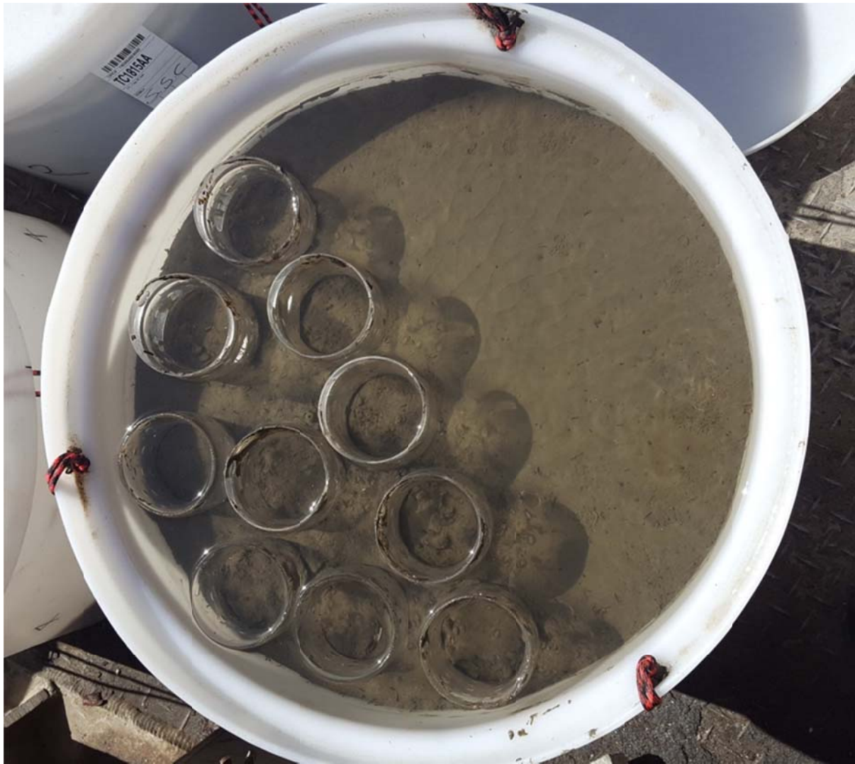
Figure 8. Control sediment cell filled with site sediment and overlying water and with pre-installed clam chambers.
