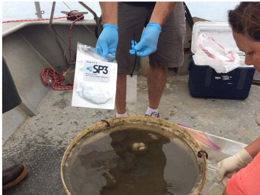
Figure 16. The SP3 polyethylene passive samplers being installed during the May 24, 2016 (T-Mid) event.
