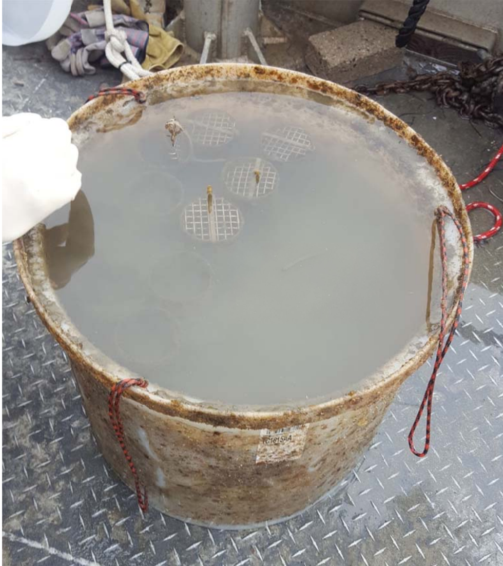
Figure 11. Preparing to remove clams and polyethylene passive samplers from a RARA sediment cell at the end of a T-Mid exposure period.
