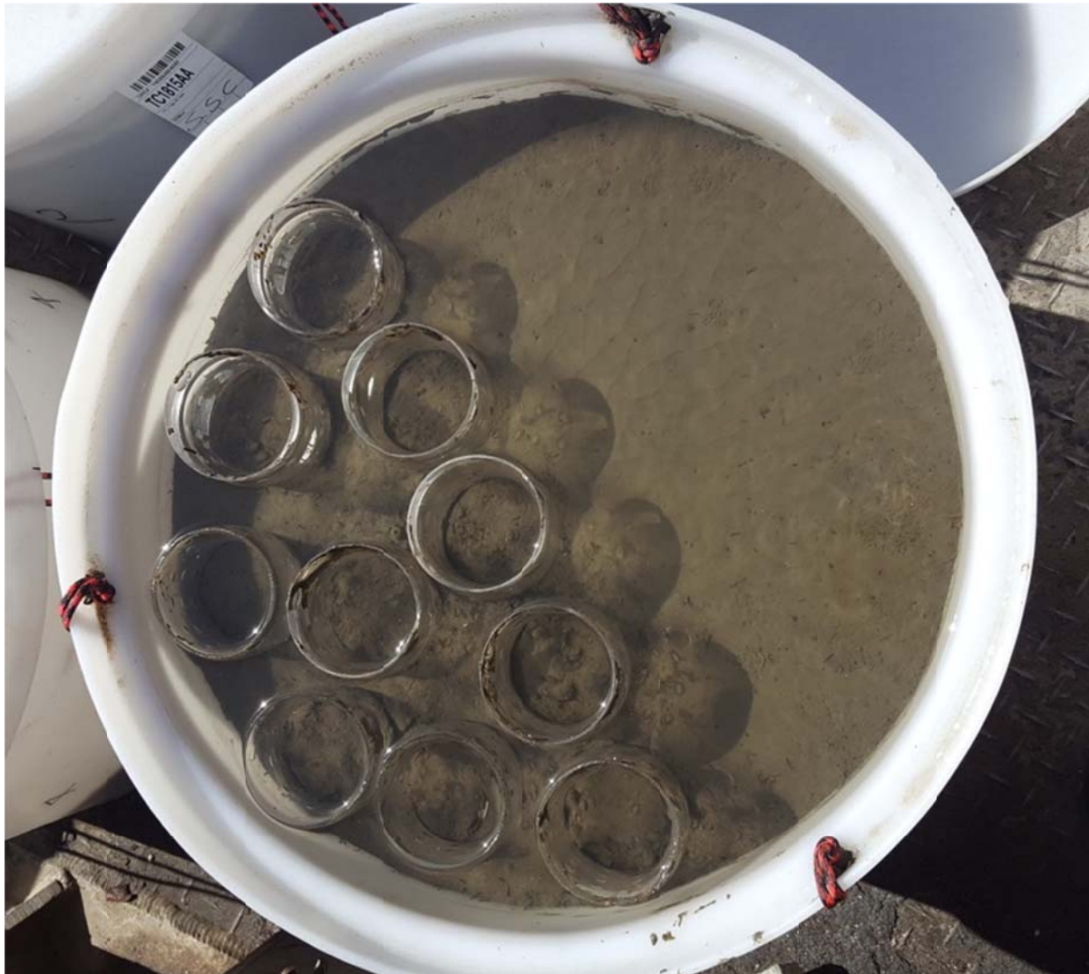
Figure 1. Control sediment cell filled with site sediment and overlying water and with pre-installed clam chambers.
