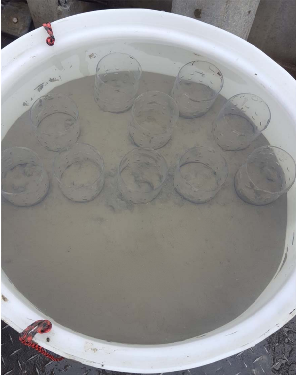
Figure 3. Final result for thin clean sediment layer treatment after final installation of treatment and overlying water.
