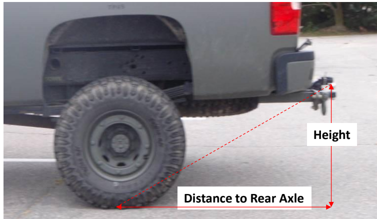
Figure 7. Prime Mover Hitch Height and Rear Axle Distance
