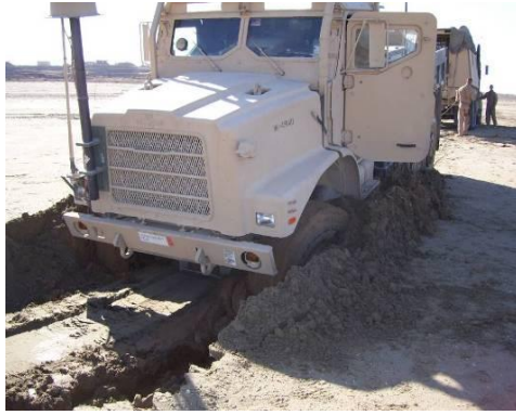
Figure 5. Soft Soils at Launch Site
