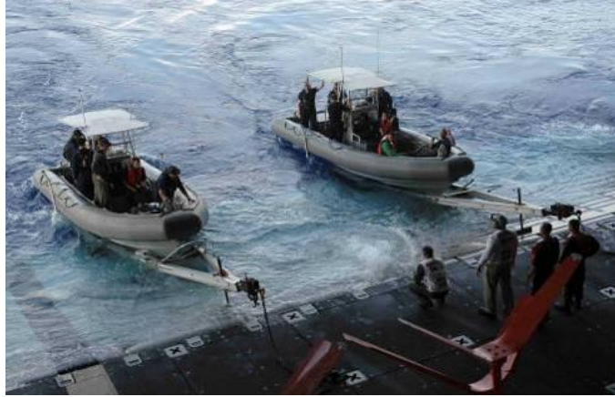
Figure 11. Stern Gate Launch and Recovery Operations
