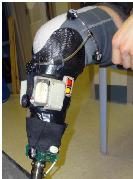
Figure 1: Assembled test prosthesis worn by a transtibial amputee.
