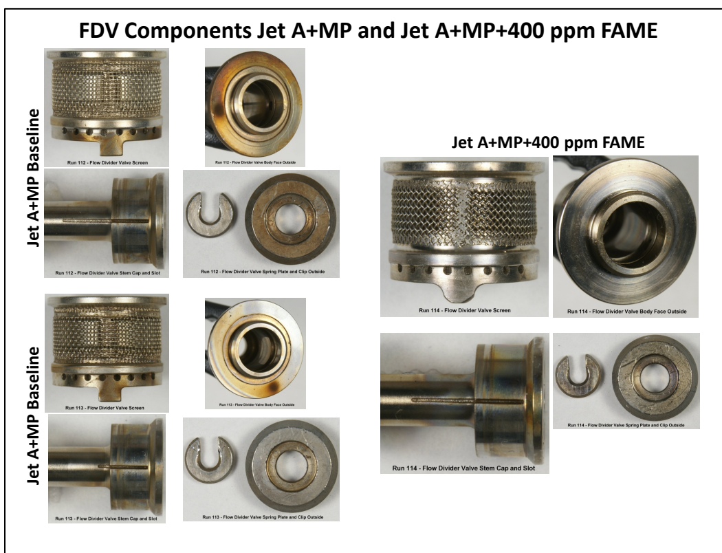
Figure 13 - Visible Deposition in FDV Components
