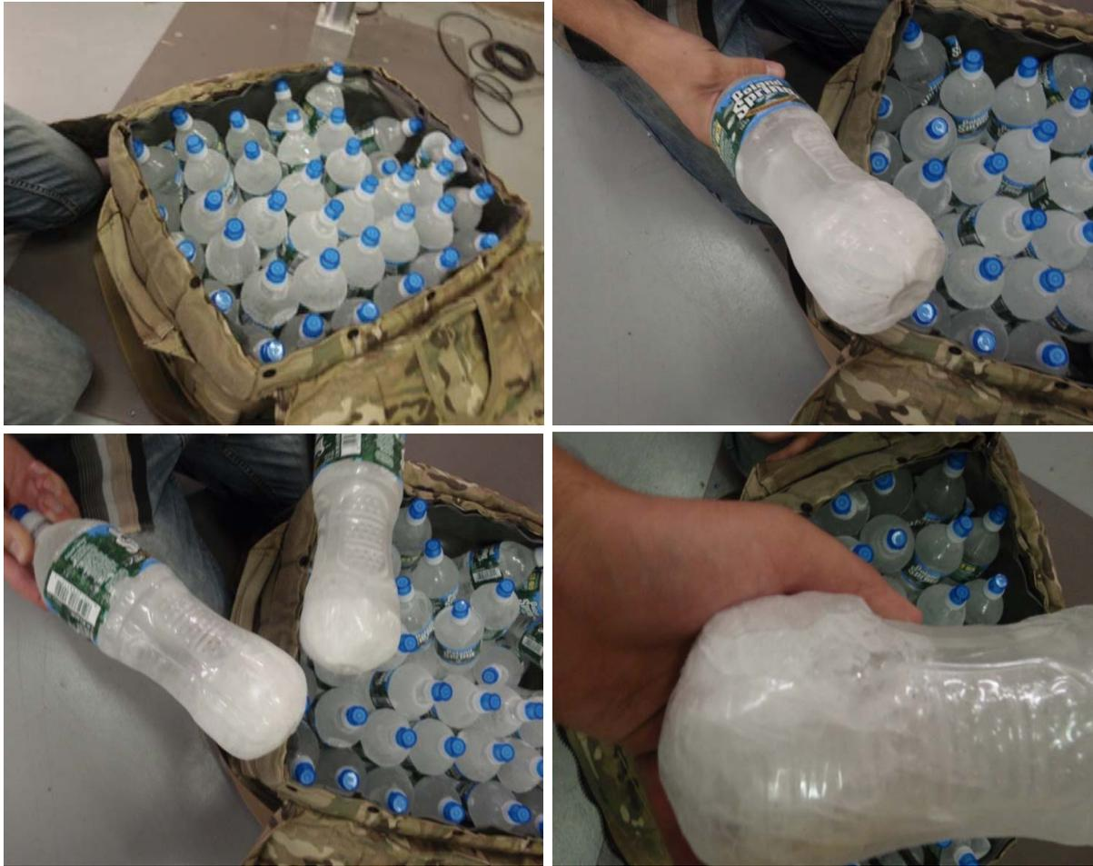
Figure 27: Large ICB Drop Test with Bag Bottom Facing Down
