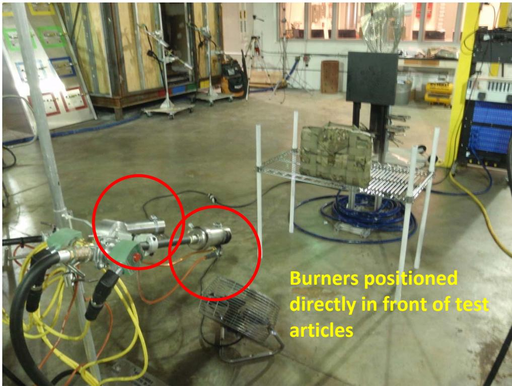
Burners positioned directly in front of test articles
