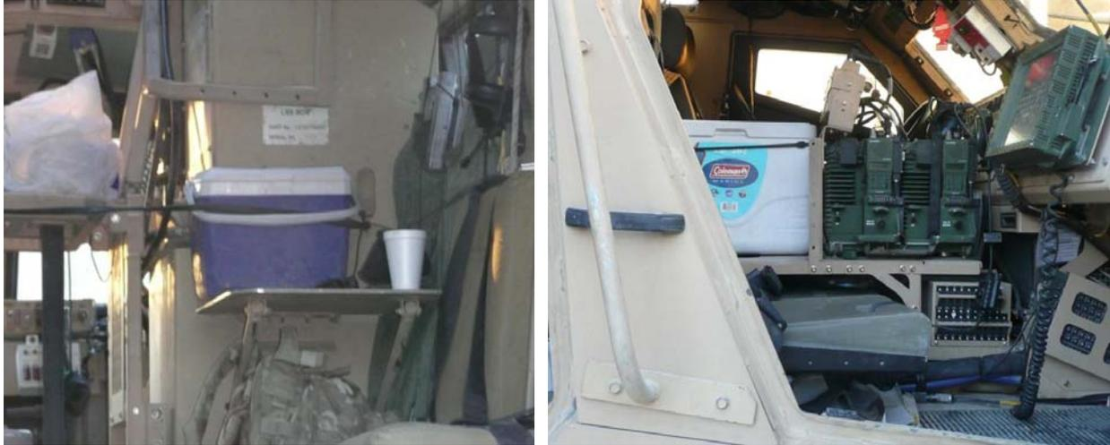
Figure 1: Ineffectively Restrained Coolers
