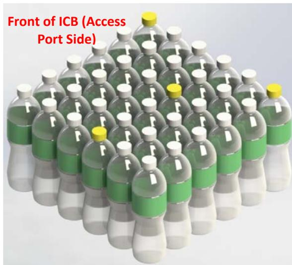
Figure 9: Large ICB Thermocouple Positions
