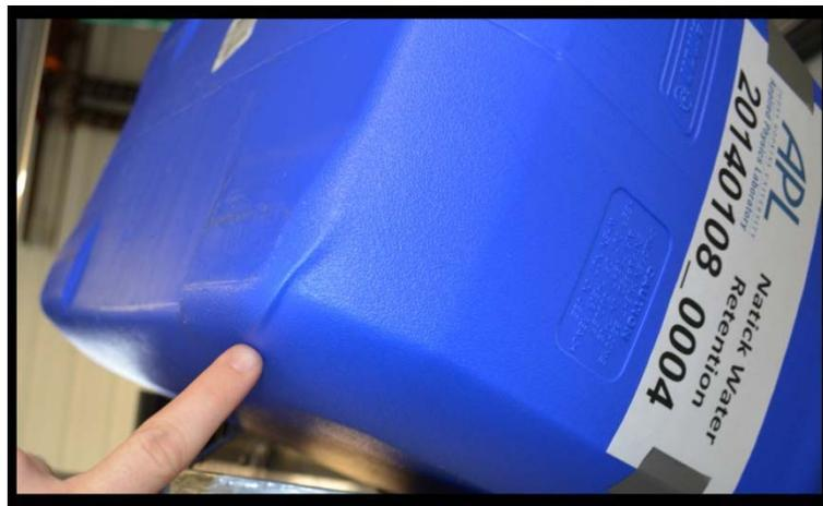
**Figure 15: COTS sustained damage at 9.0 m/s exposure**
