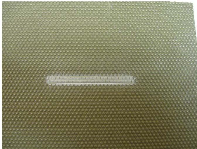
I note that the “dots” on the Superfabric wore grooves in the Wearaser. Once the “dots” were abraded through, the Wearaser abraded more on one side and wore through the fabric. EVEN if the Wearaser was refaced during the test, I do not believe the sample would have made it to 10,800 cycles
