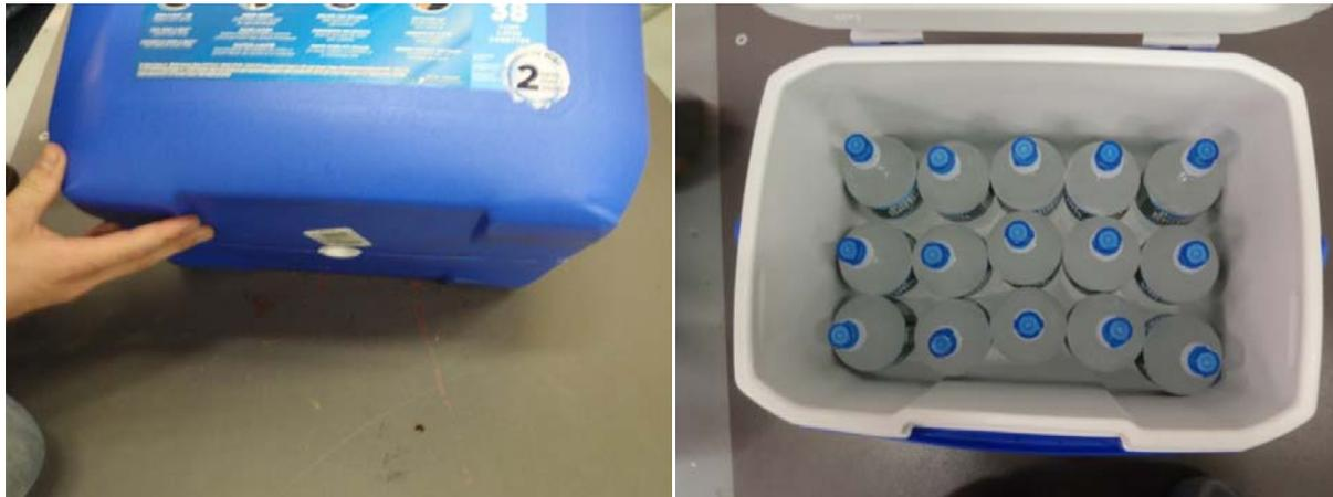
Figure 38: COTS Cooler Drop Test with Bottom Facing Down
