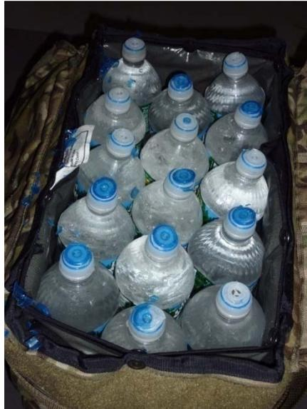
Figure 43: Aerogel ICB Drop Test with Bag Top Facing Down (Final Drop)
