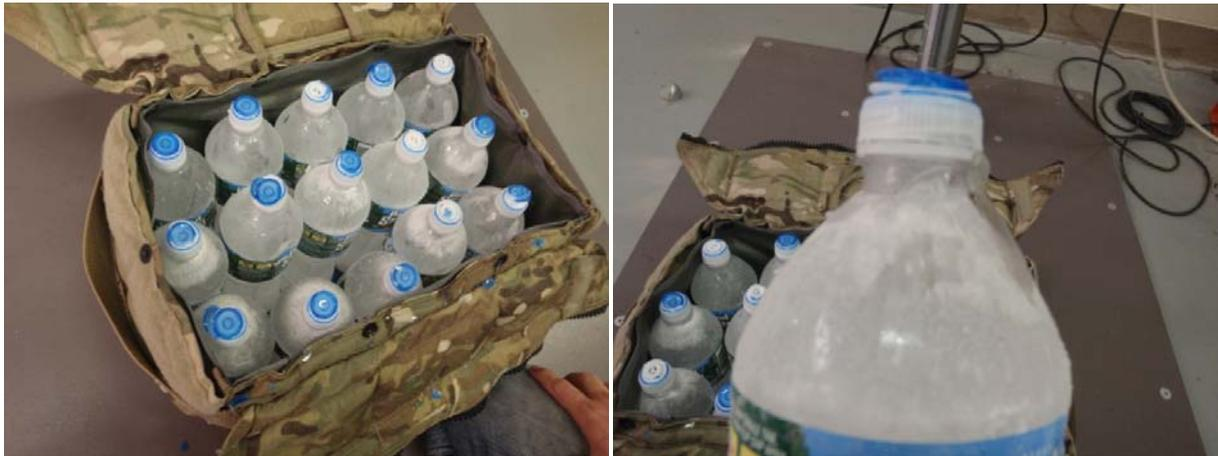
Figure 32: Medium ICB Drop Test with Bag Top Facing Down
