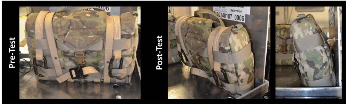
**Figure 5: Small ICB with 550 Paracord pre-test (left) and post-test (right) state**
