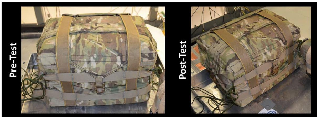
**Figure 11: Aerogel with 550 Paracord pre-test (left) and post-test (right) state**
