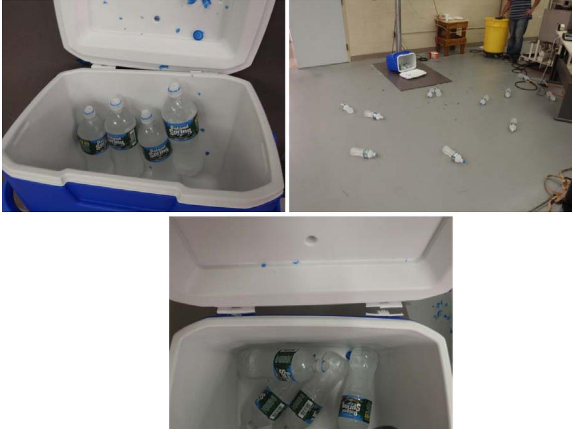
Figure 39: COTS Cooler Drop Test with Top Facing Down
