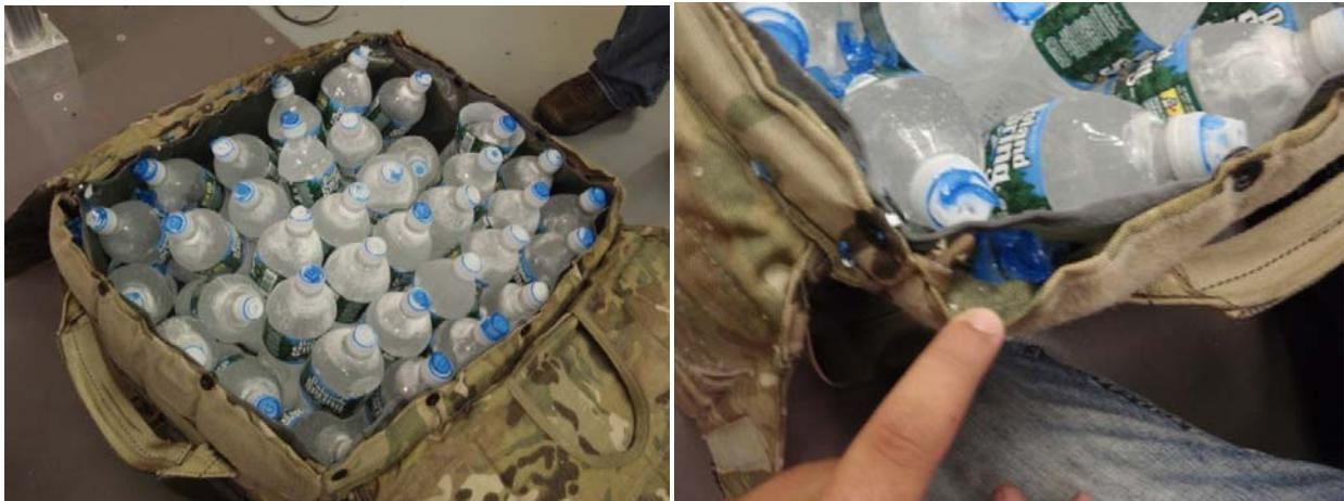
Figure 28: Large ICB Drop Test with Bag Top Facing Down
