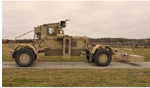
Figure 2: An early stage version of the localizing ground penetrating radar system (out front of the armored vehicle). This system steered itself based on real-time localization from the LGPR system. Operation was shown over a range of soils and road types during thousands of kilometers of operation in the US and Afghanistan.
