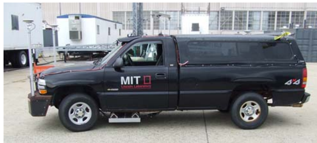
Figure 3. The low-profile LGPR system is mounted underneath the experimental vehicle. GPS/INS system antennas for the RTK truth and differential units are mounted on the outermost corners of the vehicle chassis.
