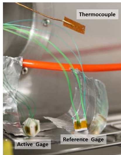
Figure 3-2: Image of thermal test set-up
