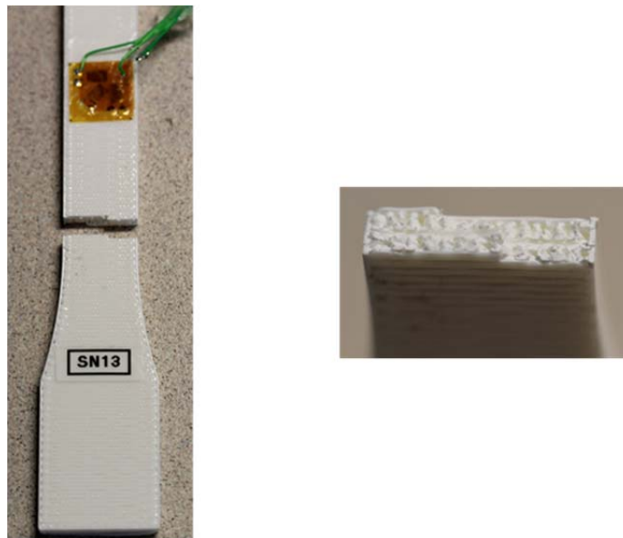
Figure 2-45 Quasi Isotropic Large Bead Test Article after destructive Tensile Testing (Left) Fracture Pattern (Right)
