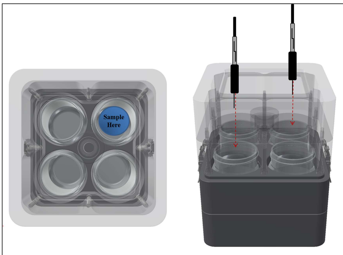
Figure 10. Diagram of experimental set-up with a single odor source in the lower portion of the LS-MODD (left) and two SPME fibers (one above from the odor and one across) at the device outlet (right).
