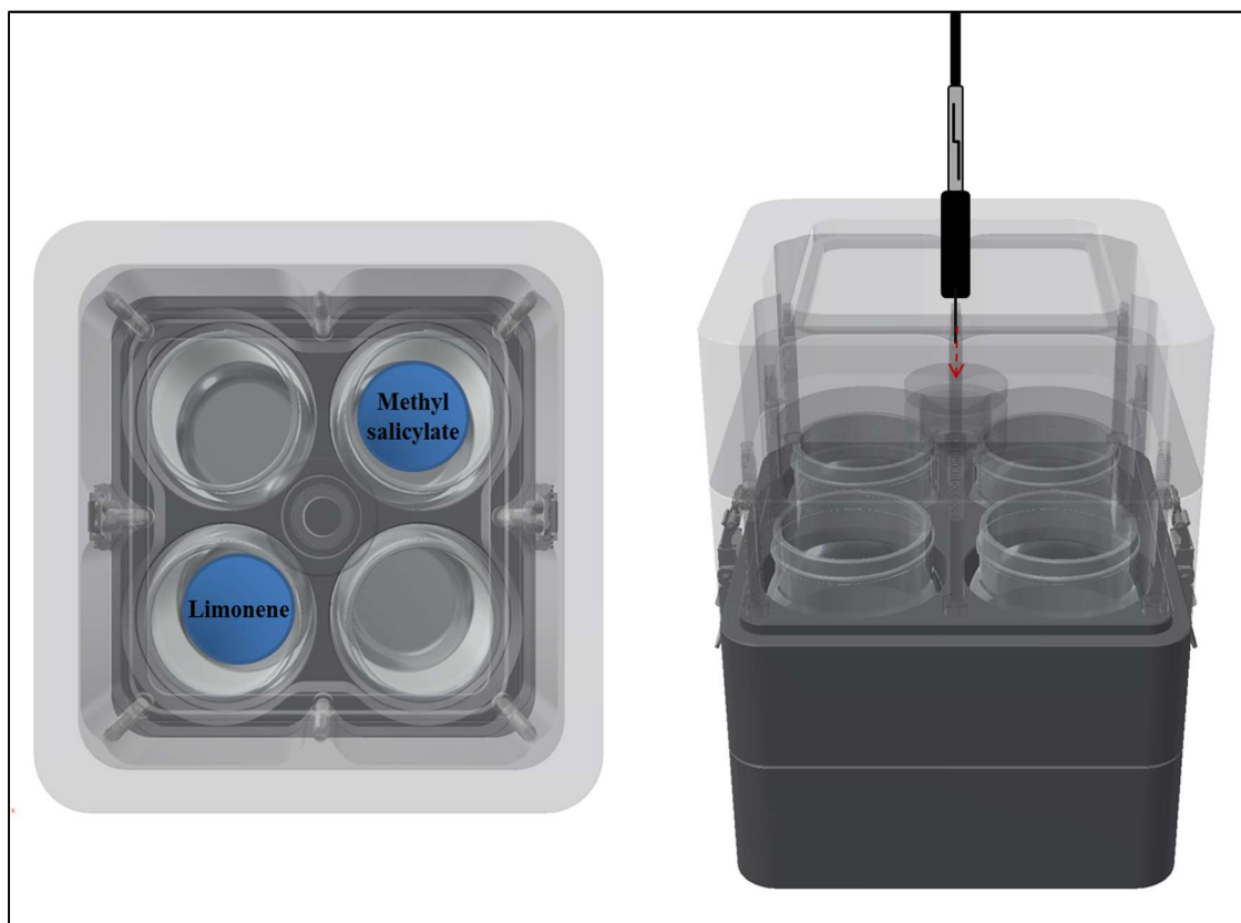
Figure 12. Diagram of experimental set-up with two odor sources in the lower portion of the LS-MODD (left) and a single SPME fibers centered at the device outlet (right).
