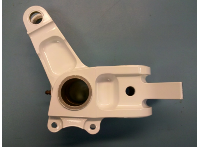
Figure 2. T-45 Pivot with Full Protective Coating System
