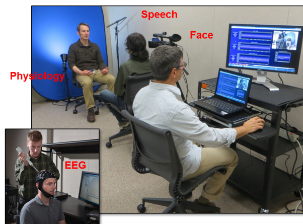
Figure 2: Multimodal platform for recording of speech, facial expression, EEG, and physiological signals.
