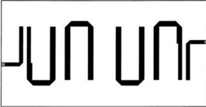
Figure 16 Hairpin resonators From (Z.-Y. Shen 2003) Linewidths are approximately  $160 \mu m$
