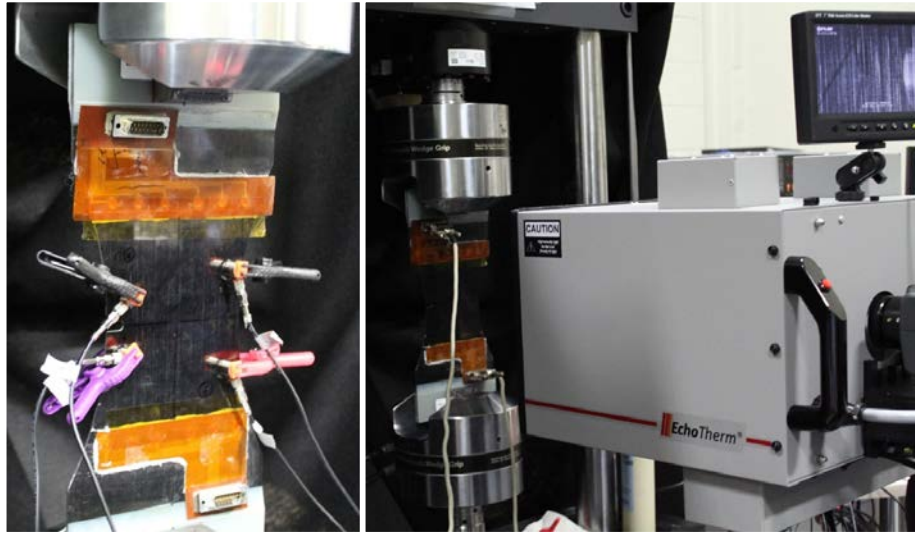
Fig. 6 Photographs showing a composite sample loaded for testing with AE sensors (left) and the thermographic imager and cables attached for ScanSentry data collection (right)
