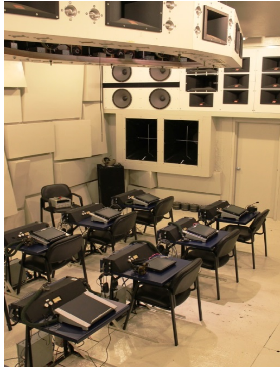
Figure 7. AFRL's VOCRES facility used to measure speech intelligibility performance
