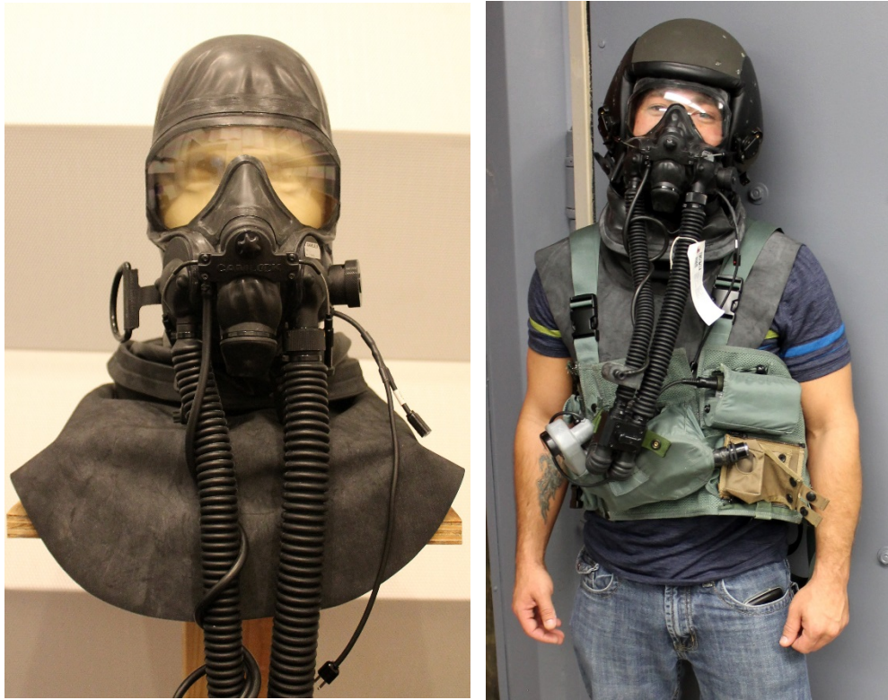
Figure 2. JSAM-TA Respirator Assembly (V)3 hood (left) and JSAM-TA Respirator Assembly (V)3 hood and torso assembly in combination with the HGU-68/P (right)
