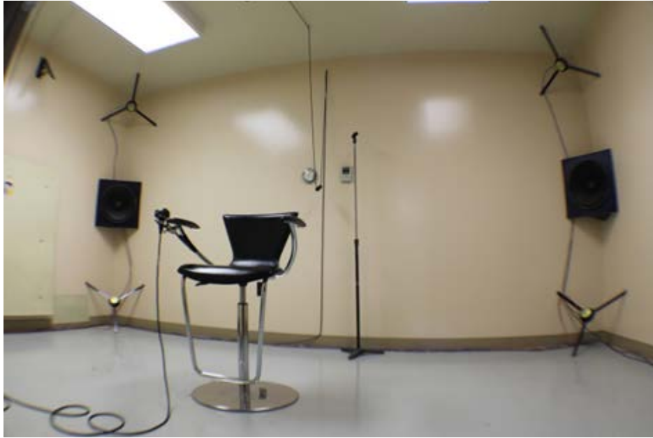
Figure 4. Facility used for measurement of passive continuous noise attenuation
