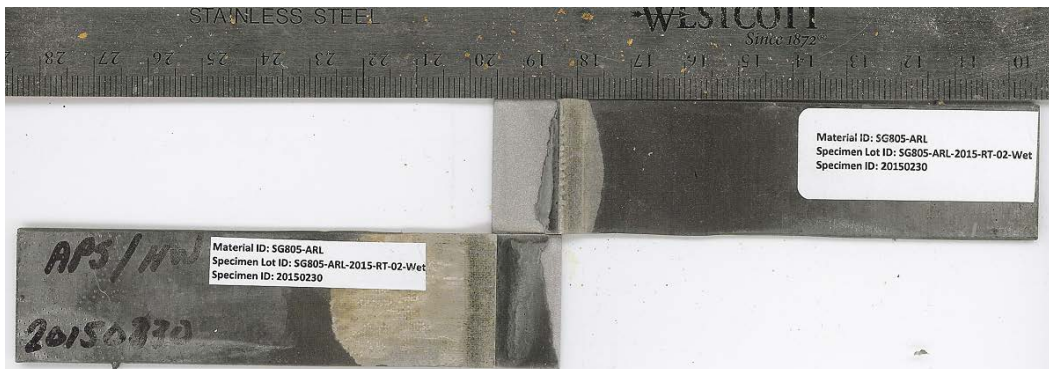
Fig. B-20 Failure surfaces for single-lap-joint with 3-aminopropyltrimethoxysilane surface pretreatment. MSAT ID = 20150230, substrate = 2024 T3 aluminum, and sample conditioning = H/W. Mode-of-failure = adhesive.
