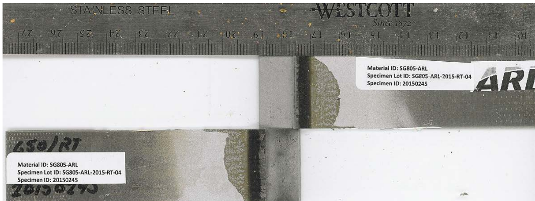
Fig. B-8 Failure surfaces for single-lap-joint with SurTec 650 surface pretreatment. MSAT ID = 20150245, substrate = 2024 T3 aluminum, and sample conditioning = RT. Mode-of-failure = MM.
