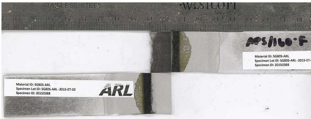
Fig. B-36 Failure surfaces for single-lap-joint with 3-aminopropyltrimethoxysilane pretreatment. MSAT ID = 20150388, substrate = 2024 T3 aluminum, and test conditions = ET Mode-of-failure = adhesive.
