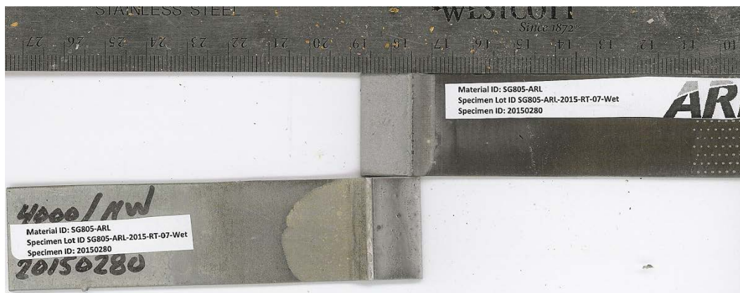
Fig. B-30 Failure surfaces for single-lap-joint with XBOND 4000DM-DR surface pretreatment. MSAT ID = 20150280, substrate = 2024 T3 aluminum, and sample conditioning = H/W. Mode-of-failure = adhesive/ MM.
