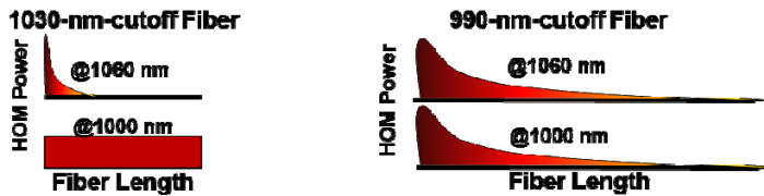
Fig 3. HOM power decay along fiber length for 2 fibers with same 17- \mu m MFD but different cutoff wavelengths. Different fiber waveguide designs are used to achieve the cutoff wavelengths. The fiber with shorter cutoff wavelength can have slower HOM decay at 1060 nm operating wavelength.
