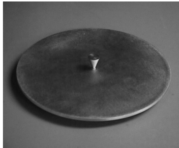
Figure 4.13 Photograph of a conical monopole over a circular ground plane, designed for the 3.1 to 10.6 GHz band (prototype 1).
