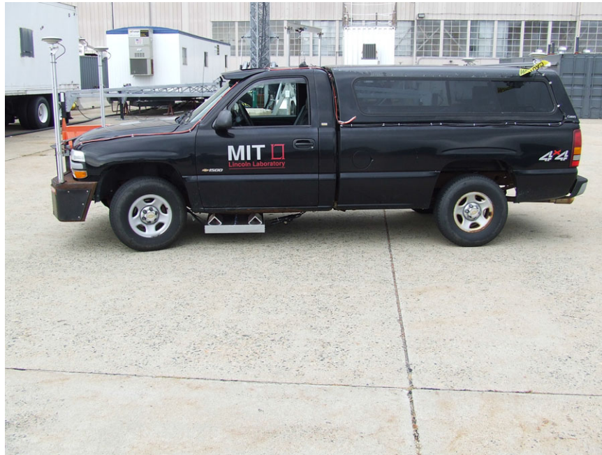
Figure 3. The low-profile LGPR system is mounted underneath the experimental vehicle. GPS/INS system antennas for the RTK truth and differential units are mounted on the outermost corners of the vehicle chassis.
