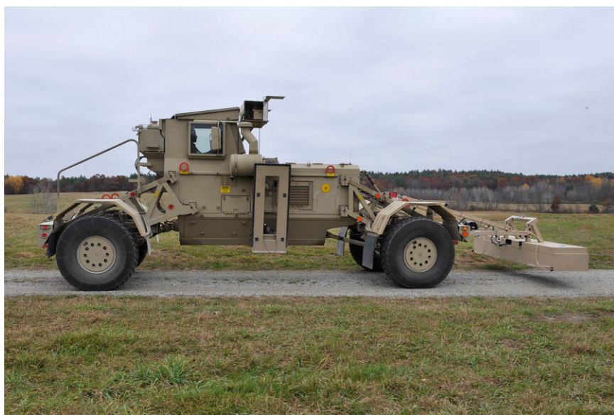
Figure 2. An early-stage version of LGPR (out front of the armored vehicle). This system steered itself based on real-time localization from the LGPR system. Operation was shown over a range of soils and road types during thousands of kilometers of operation in the United States and Afghanistan.
