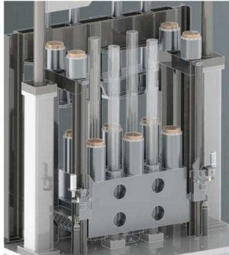
Figure 5: VALTS Guided Ballistic Masses
