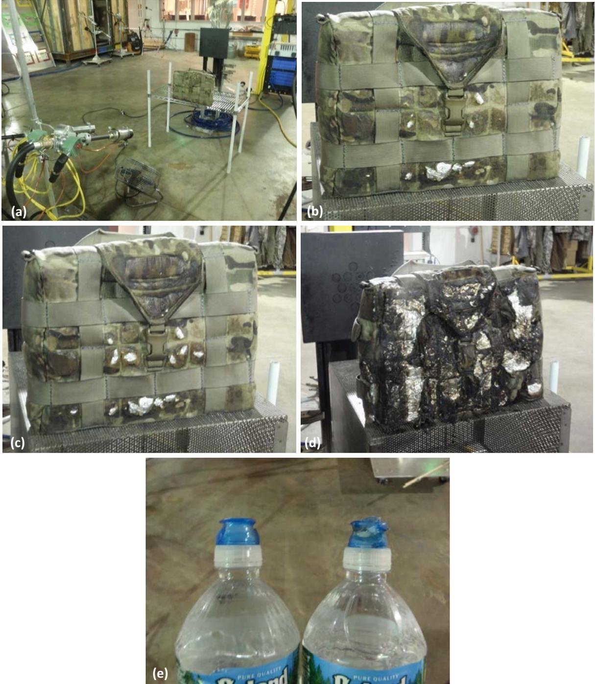
Figure 52: Small ICB Flash Oil Fire Test Results: (a) Test Setup; (b) After Initial 4-s Burn; (c) After Second 4-s Burn; (d) After Final 10-s Burn; (e) Damage on Bottles after 10-s Burn
