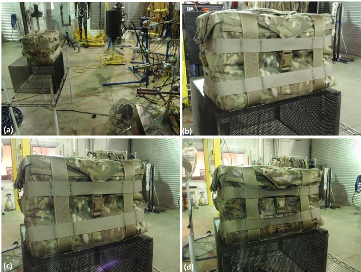
Figure 54 Aerosol ICB Flash Oil Fire Test Results: (a) Test Setup; (b) After Initial 4-s Burn; (c) After Second 4-s Burn; (d) After Final 10 s Burn
