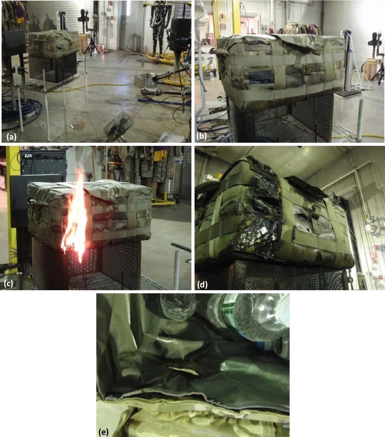
Figure 55: Large ICB Flash Oil Fire Test Results: (a) Test Setup; (b) After Initial 4-s Burn; (c) Sustained Ignition During Second 4-s Burn; (d) After Second 4-s Burn; (e) Interior after Second 4-s Burn
