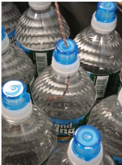
Figure 7: Thermocouple Installation into Water Bottles
