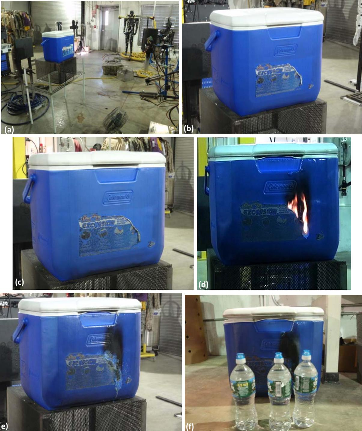
Figure 56: COTS Cooler Flash Oil Fire Test Results: (a) Test Setup; (b) After Initial 4-s Burn; (c) After Second 4-s Burn; (d) Sustained Ignition during 10-s Burn; (e) After 10-s Burn; (f) Undamaged Bottles with Damaged COTS Cooler after 10-s Burn
