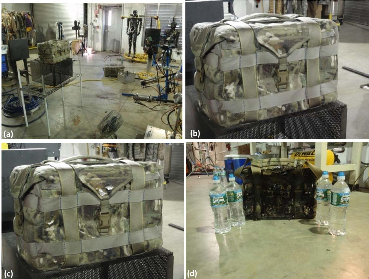
Figure 53: Medium ICB Flash Oil Fire Test Results: (a) Test Setup; (b) After Initial 4-s Burn; (c) After Second 4-s Burn; (d) After Final 10-s Burn
