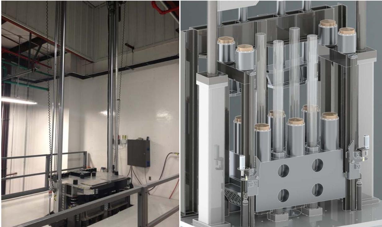
Figure 2: Vertically Accelerated Load Transfer System (VALTS), Bullet mass assembly and pulse shaping elastomers (Left), mounting table and guide rods (Right). The bullet is accelerated upwards to strike the table which rides along the two vertical guide rods inducing controllable levels of UBB exposure.
