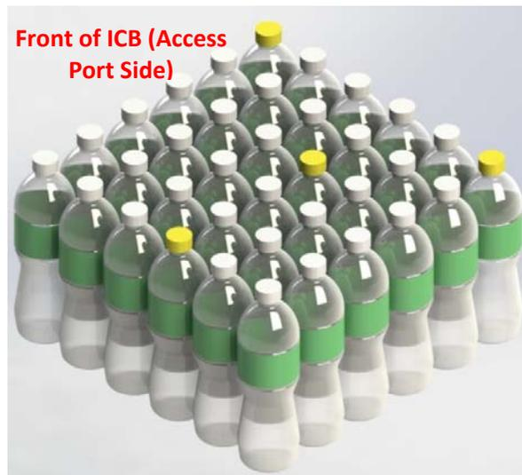
Figure 9: Large ICB Thermocouple Positions
