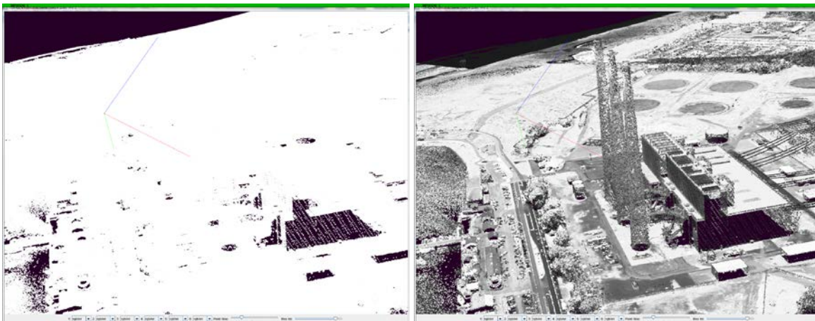
Figure 2 - Left, a point cloud colored only in white; right, the same point cloud colored with its intensity values. Coloring and shading makes all the difference in understanding the structure of dense point clouds.
