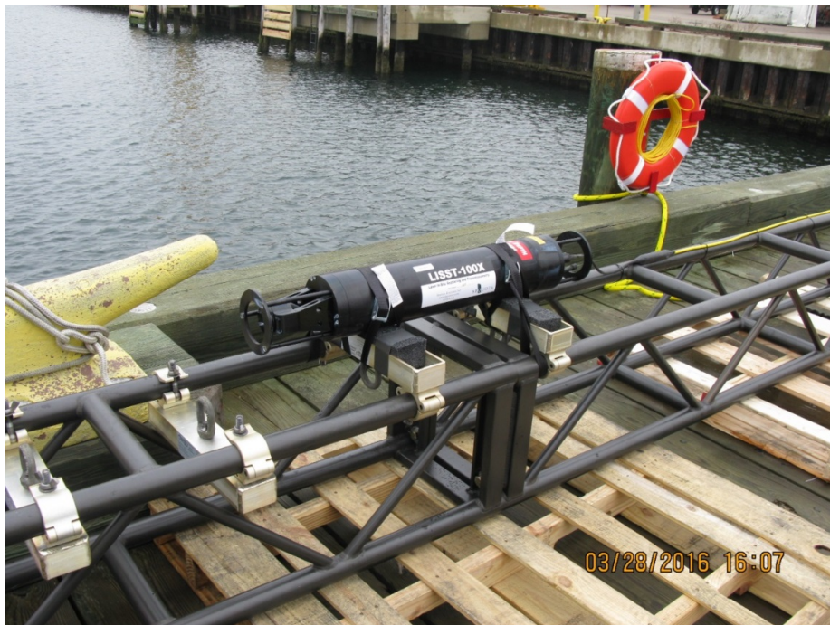
Figure 16. LISST-100X mounted to the truss assembly.
