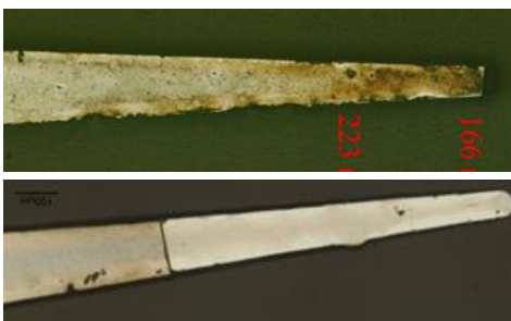
Figure 3: Optical etched micrograph showing amorphous tip of Al_{40}Mg_{40}Ga_{15}Ca_5 and amorphous skin of Al_{45}Mg_{40}Ga_{10}Ca_5
