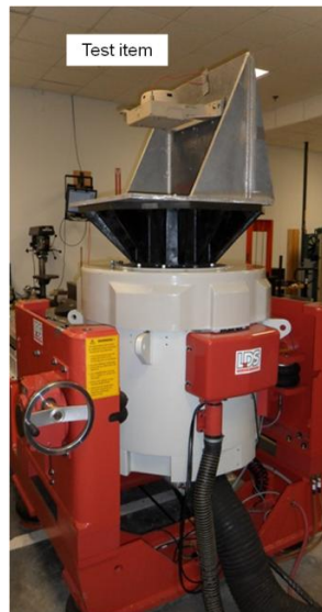
Figure 1. Example Laboratory Shock and Vibration Machine 1
