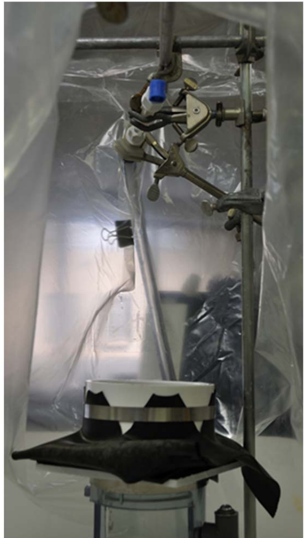
Close-up of the spray chamber, showing the spray nozzle (blue, top) and the screen support holding the Comp B residues (bottom).
