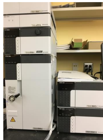
Figure 4. Gel permeation chromatography (GPC) that runs DMF as mobile phase from Shimadzu.
