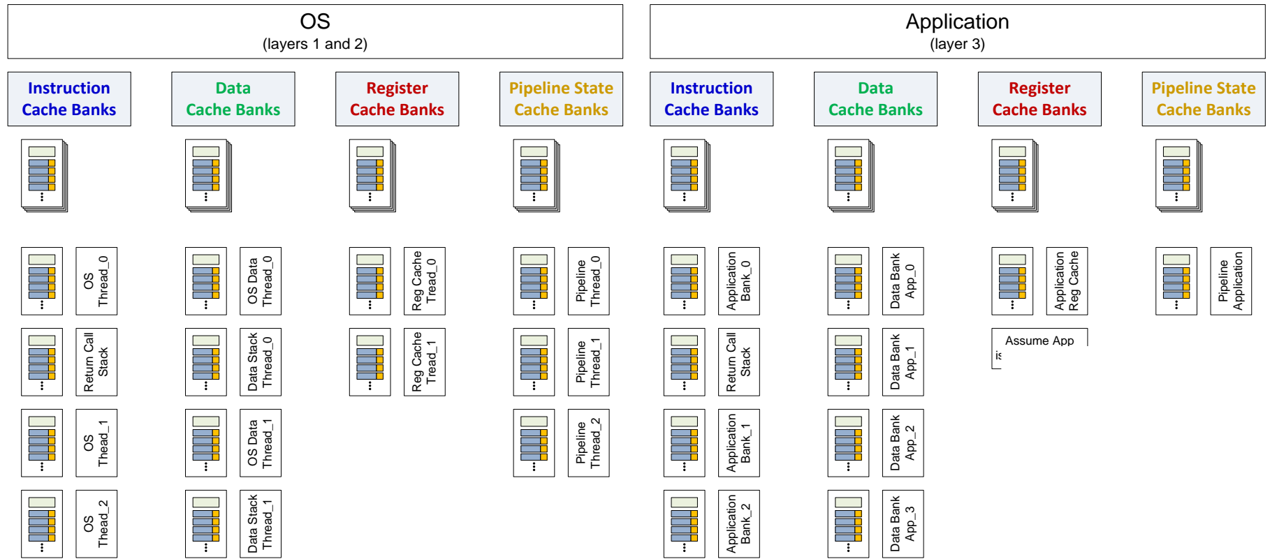
Fig. 27 OS and application cache bank organization
