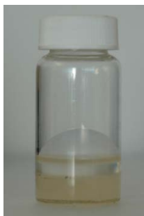
Fig. 159 Photograph showing insolubility of UPE1/styrene (70/30)
