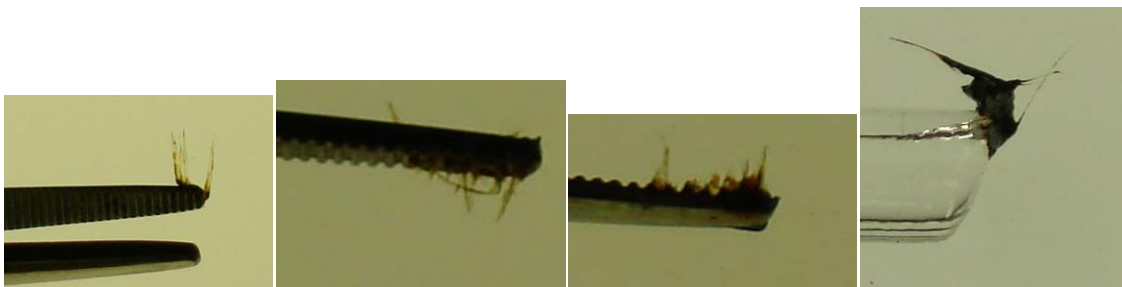
Fig. 39 Tweezer stretching experiment of scaled-up Pseudomonas decomposed lignin sample
