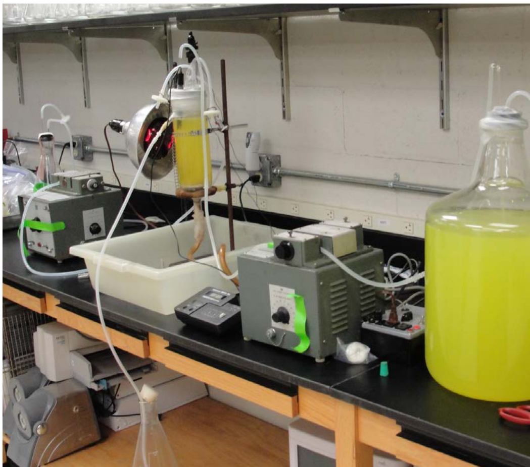
Fig. 9 Chemostat assembled for lignolytic microorganism isolation
