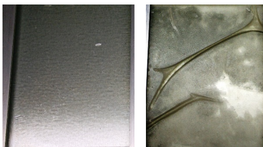
Fig. 178 Commercial coating (left) and isosorbide coating (right) after QUV exposure
