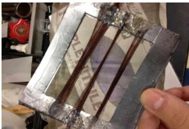
Fig. 87 Mounted fibers on graphite frame
