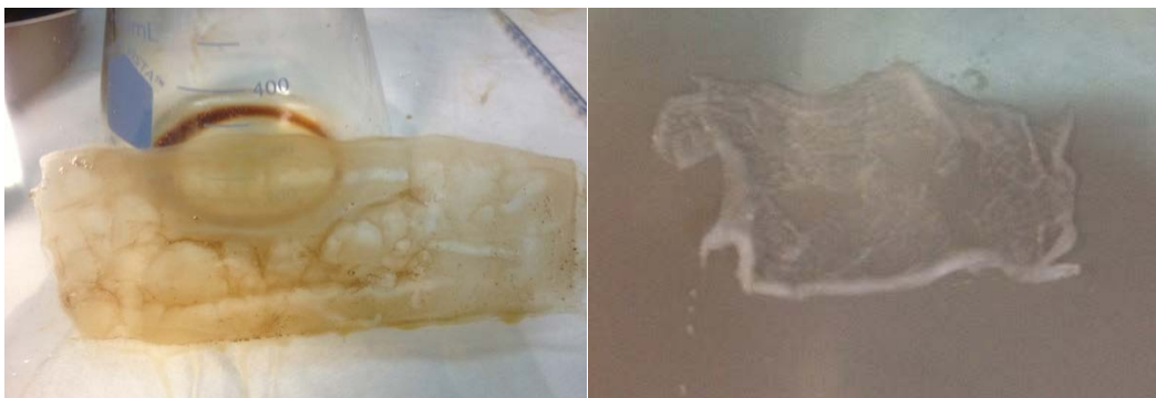
Fig. 106 Comparison of dilute PFA and PAN solution after coagulation
