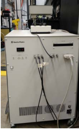
Figure 3.32: PIV laser power supply (foreground) and laser system (background)
