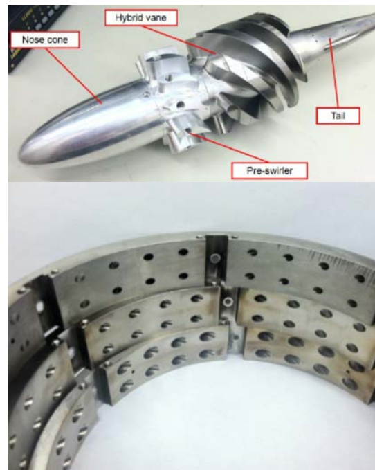
Figure 2.63: Full annular center section hardware (top) and air/fuel injection rings with varying diameters (bottom) [90]
