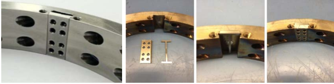
Figure 2.64: Installed fuel baffle (left-most image); installation of fuel baffle addition (right three images)
