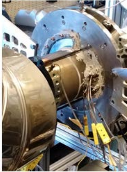
Figure 3.21: Extended exhaust cowling for PIV/PSEV testing
