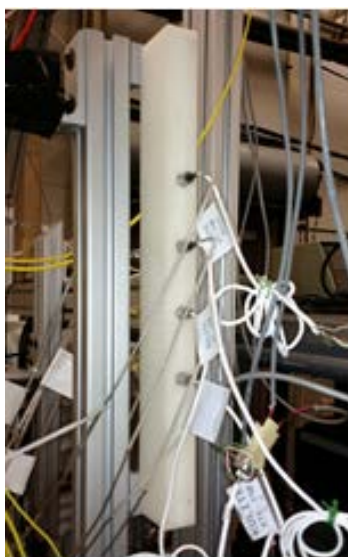
Figure 3.26: Kulite probe installation
