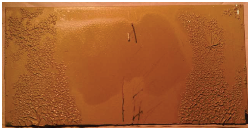
Figure 16. Old panel exposed to condensed vapors from 0.10 vol % DiEGME in the bulk fuel.
