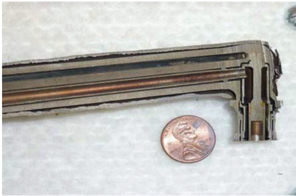
Fig. 1 Image of sectioned fuel nozzle.
