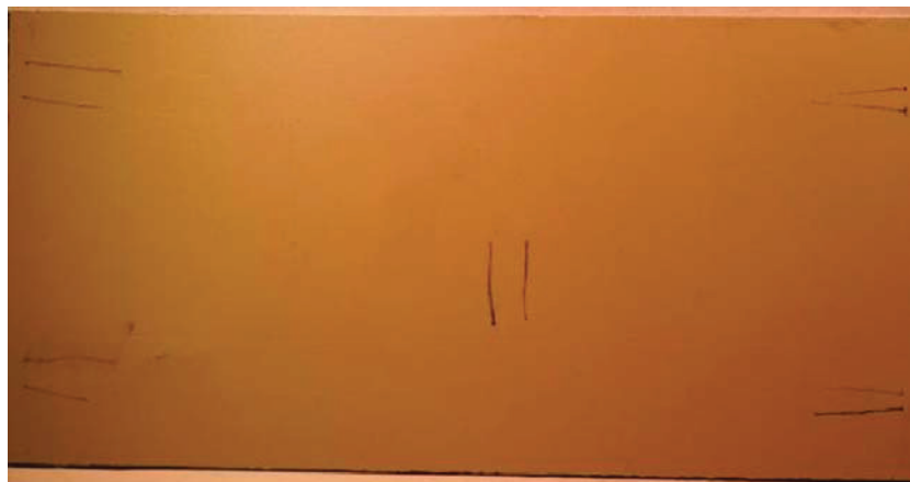
Figure 14. Old panel exposed to condensed vapors from 0.05 vol % DiEGME in the bulk fuel.
