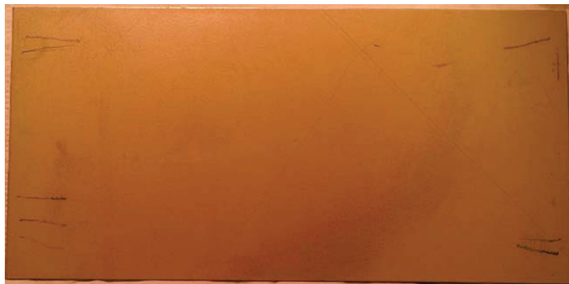
Figure 17. Old panel exposed to condensed vapors from 0.10 vol % TriEGME in the bulk fuel.
