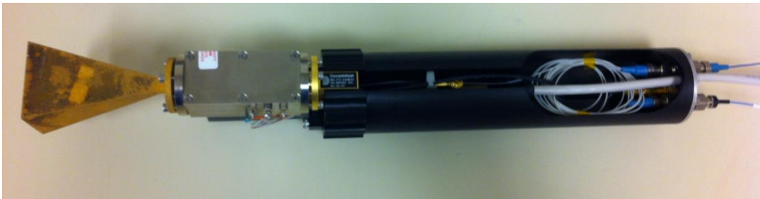
Figure 20. RF Front-End Module in current Pathfinder imaging receiver demonstration system with a length of ~14" and a 3" diameter with protrusions that set the minimum pitch of the array to ~4". From left two right, components of chain include horn antenna, waveguide based low noise amplifier, and COTS optical modulator embedded in plastic holding cylinder.
