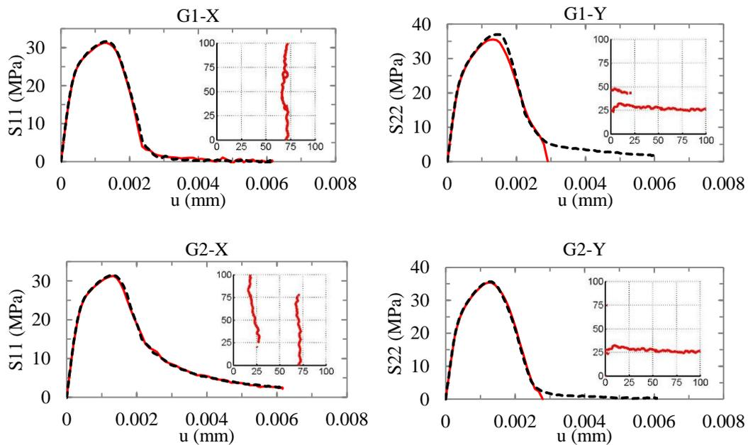
Figure 5. Comparison of simulation results using the multi-scale stochastic coupling strategy for weak interface properties. The solid curves represent the detailed geometry models (i.e. MeE size  $100\mu\text{m}^2$ ) and dashed curves are the Bayes multi-scale models.
