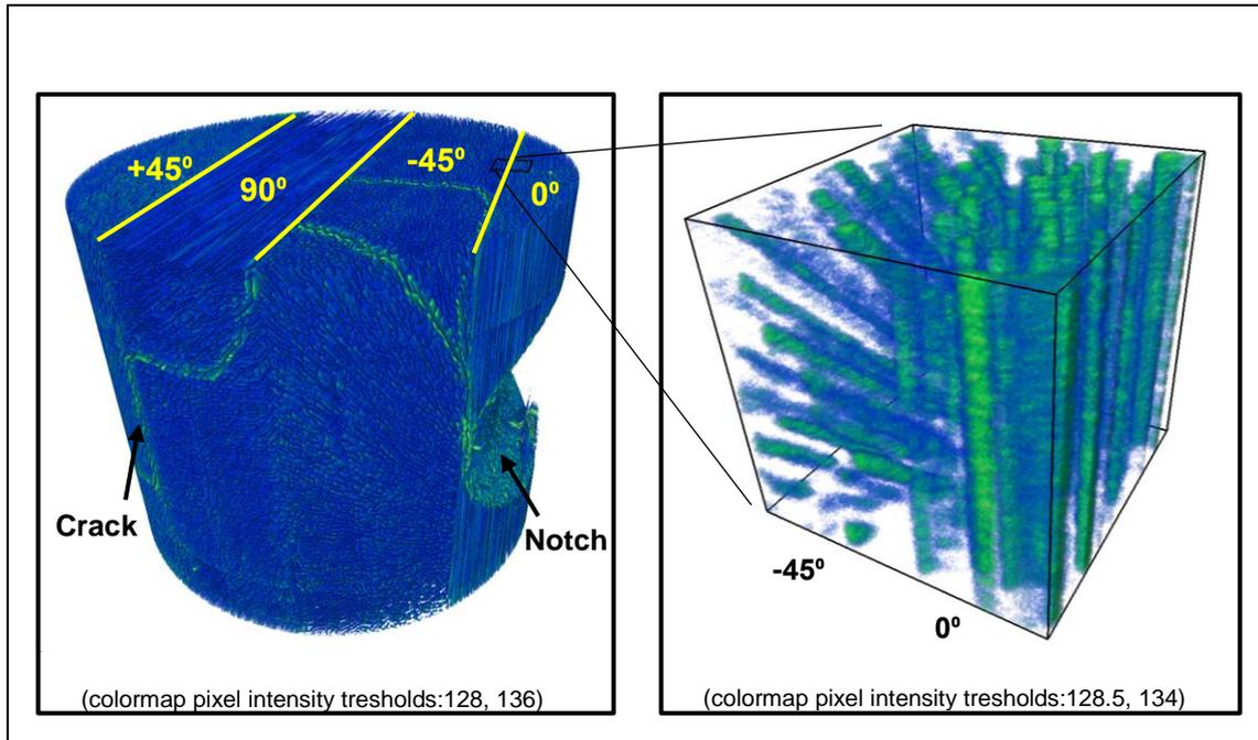
Figure 2: An X-ray CT volume render of the cross-ply CFRP
