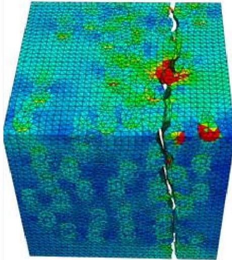
Figure 6. 3D cohesive fracture modelling of CFRP
