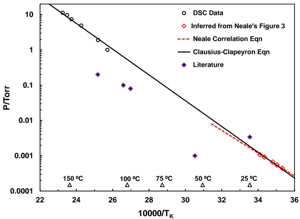
Figure 6. IMPA vapor pressure data and Clausius–Clapeyron correlations.
