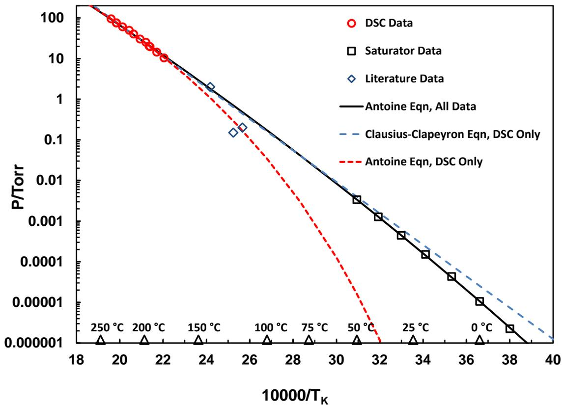
Figure 3. DCMP vapor pressure data and Antoine correlations based on all data and DSC data only, and the Clausius–Clapeyron equation based on DSC data only.
