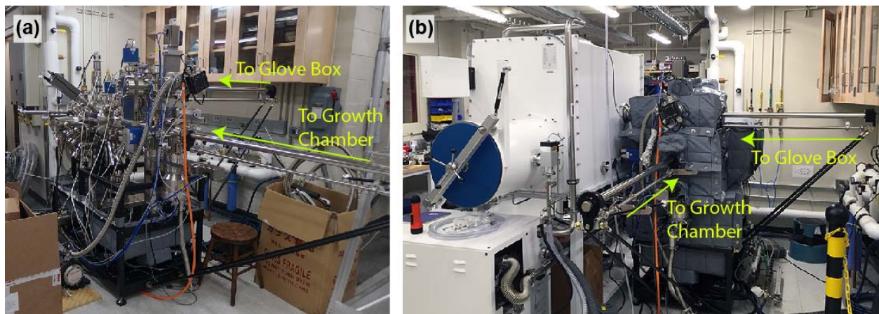
Figure 1 – (a) Molecular Beam Epitaxy (MBE) chamber before glove box attachment. Manipulator arms to connect to the growth chamber and glove box are labeled. (b) MBE chamber after glove box attachment (rotated view). The same manipulator arms are labeled. In this image heating blankets are attached to the MBE.
