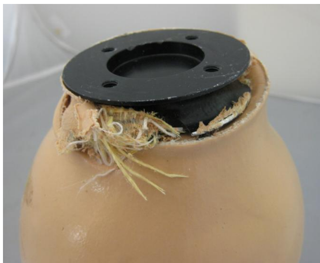
Figure 3: NU-1 distal adapter failure
