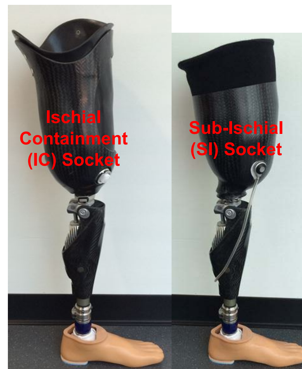
Figure 2. Ischial containment socket with passive suction suspension on left and sub-ischial socket with vacuum-assisted socket suspension on right. Both sockets worn with a gel liner, X3 microprocessor knee and energy storage and return foot.
