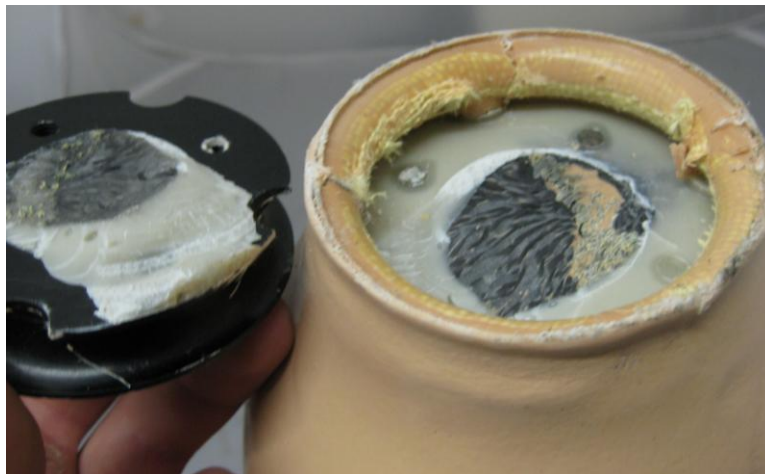
Figure 5: NU-3 distal adapter failure
