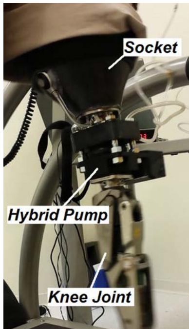
Fig. 3 Location of the hybrid vacuum pump for use within a transfemoral prosthesis. Pyramid adaptors fixed to proximal and distal ends of the pump housing were used for installation of the pump between the socket and knee joint, respectively.
