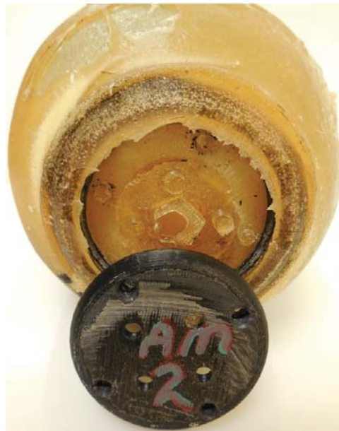
Figure 2.8. Failed distal adapter on tested AM socket
