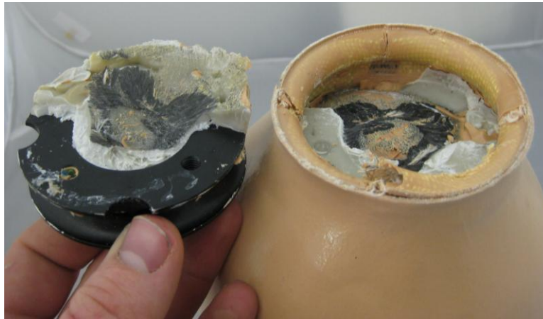
Figure 4: NU-2 distal adapter failure
