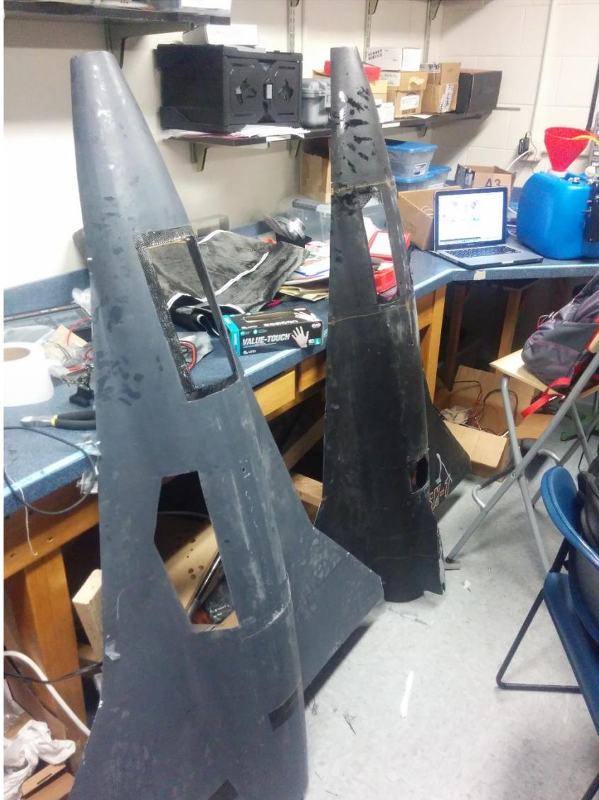
*Figure 18: Shows the skin with doors and panels cut out*
