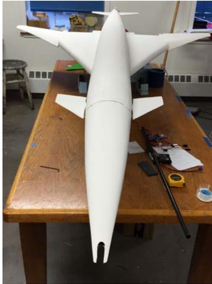
Figure 10: The 2015 UW UAV without vertical tail and boom
